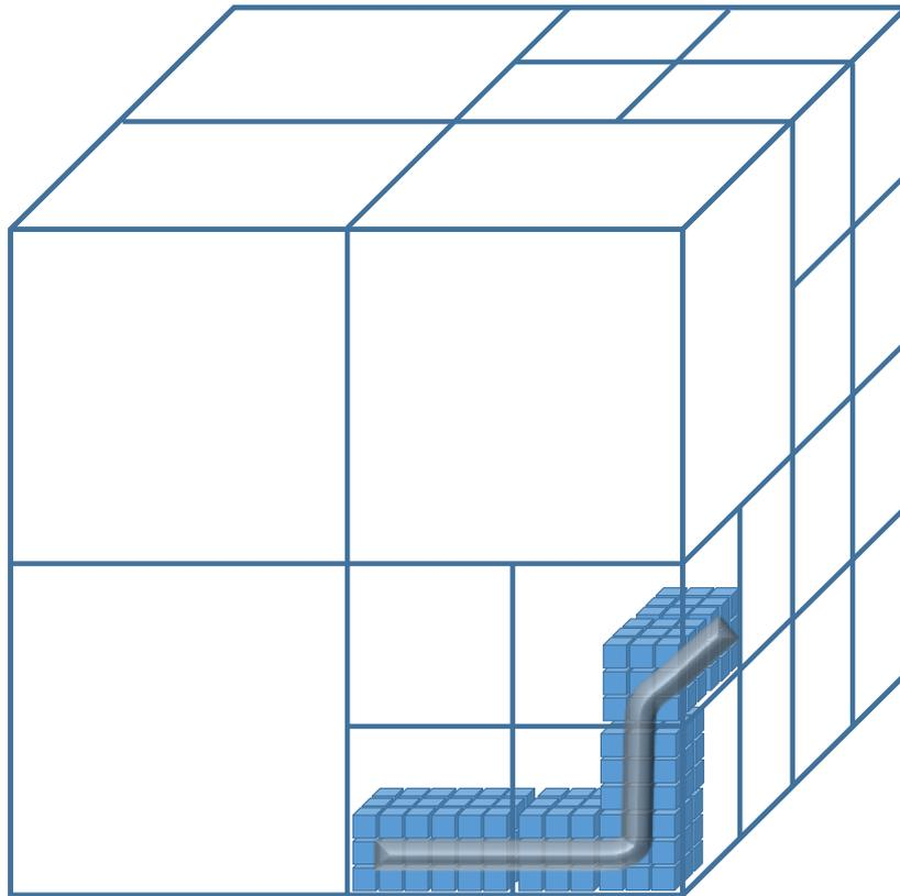
Figure 6: *Hybrid octree* optimized for likelihood field storage. The grey pipe storage is split in two parts. First, the octree is computed for a resolution  $R_o$ . Secondly, a 3D occupancy grid is used to store finer resolutions up to resolution  $R_a$ . As it can be seen in Table 1, the memory size is significantly reduced compared to a regular octree structure when applied to dense data such as likelihood fields
