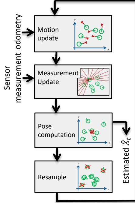
Figure 2: Main steps of particle filter-based localization
