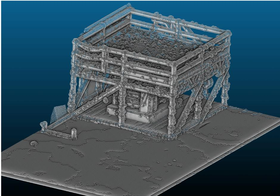
Figure 4: 3D representation of the environment stored by the octree (Figure 14a). Only regions where the likelihood is larger than zero are represented. Storage size of the likelihood : 8 bits,  $\sigma_{map} = 3cm$ . The likelihood field presented is the map used in our experiments
