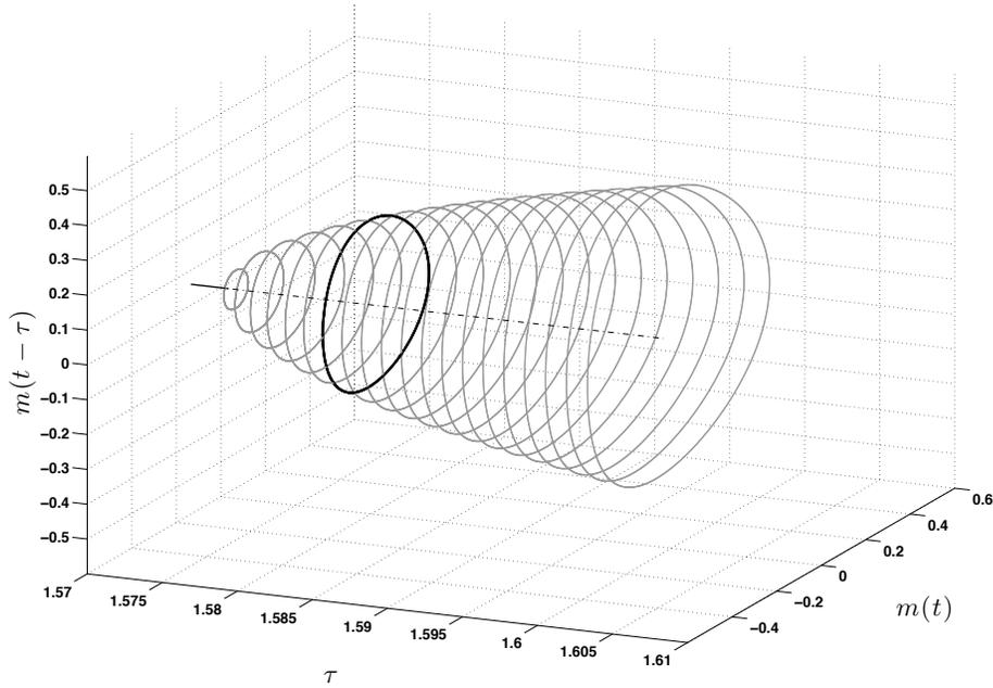
FIGURE 1. Unfolding of the Hopf bifurcation taking place for Eq. (3.1) as  $\tau$  is varied. The limit cycles are represented in the embedded reduced phase space  $(m(t), m(t - \tau))$ . The limit cycle in heavy black indicates the “ $\tau$ -section” considered for the numerical results of Sectns. 3.3 and 4 below. The trivial steady state is represented via a dotted line when unstable and a plain one when stable.
