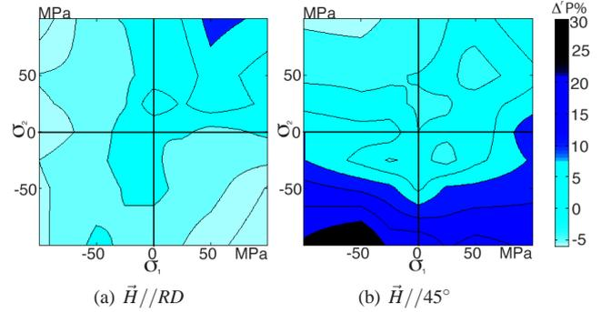
Fig. 4. Relative variation  $\Delta^r P$  of the power losses in the stress plane for a magnetic loading along RD (a) and at  $45^\circ$  (b) -  $f=5\text{Hz}$ .
