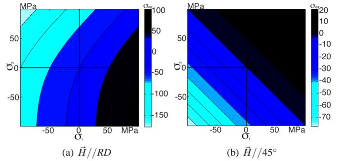
Fig. 5. Equivalent stress  $\sigma_{eq}$  in the stress plane.
