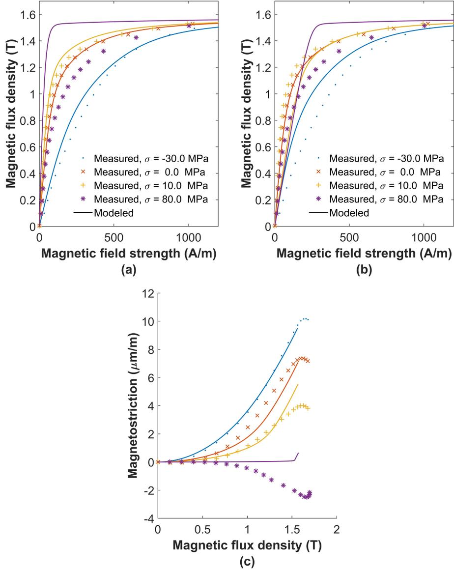
Figure 4: Comparison of measured uniaxial stress dependent anhysteretic magnetization and magnetostriction with modeled results from SM model. (a) Anhysteretic magnetization results without  $H_{\text{conf}}$  ( $\eta = 0$ ). (b) Anhysteretic magnetization with  $H_{\text{conf}}$  ( $\eta = 2.33 \cdot 10^{-4}$ ). (c) Anhysteretic magnetostriction results. (Same legend as in Fig. 4. (a) and (b))
