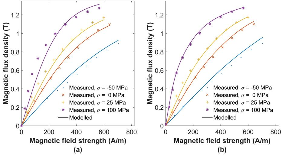
Figure 1: Comparison of measured uniaxial stress dependent anhysteretic magnetization results with modeled results from (a) SM model and (b) HE model.
