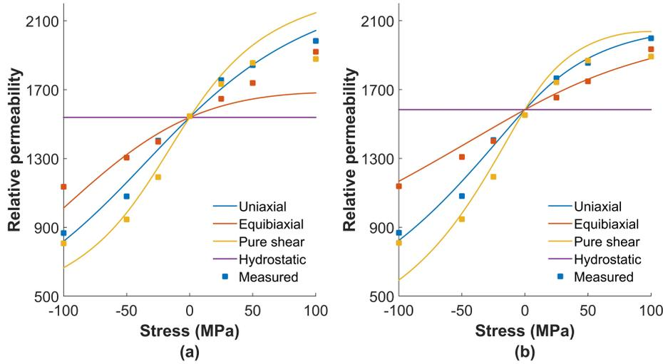
Figure 2: Permeability evolution under multiaxial magneto-mechanical loadings for Material I. Measured permeabilities are shown with the markers. Results obtained from (a) the SM model and (b) the HE model.
