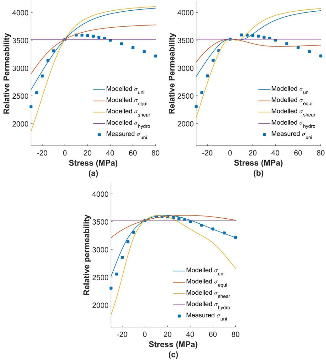
Figure 7: Permeability evolution under multiaxial magneto-mechanical loadings for Material II. Measured uniaxial permeabilities are shown with the markers. (a) SM model results without  $\mathbf{H}_{conf}$  ( $\eta = 0$ ), (b) SM model results with  $\mathbf{H}_{conf}$  ( $\eta = 2.33 \cdot 10^{-4}$ ), (c) HE model results.
