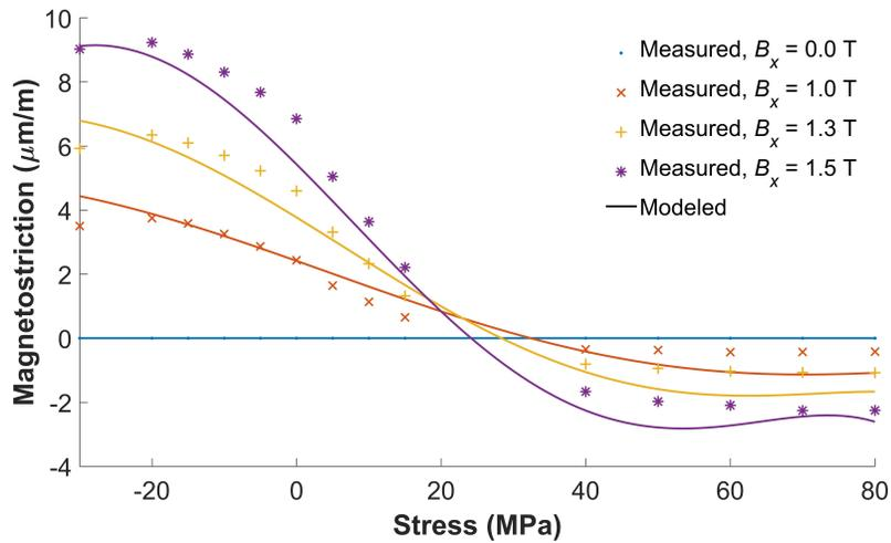
Figure 6: Comparison between modeled and measured uniaxial stress depended magnetostriction under several induction levels applied along rolling direction ( $x$ ) for Material II. Modeling results are obtained from the HE model.
