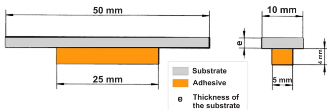
Fig. 1. Dimensions of the sample, in accordance with ISO Standard 14679 – 1997 [19].
