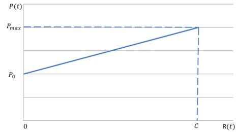
Fig. 1. Power model of a network's equipment.
