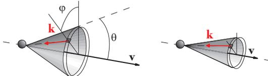
FIG. 2. (Color online) Auto-adaptation of the resonance condition for an atom with velocity  $\mathbf{v}$  in presence of isotropic light. When the atom slows down due to the absorption of photons with wave vectors  $\mathbf{k}$ , the cone fulfilling the Doppler resonance condition closes, being fully closed for  $v = |\Delta|/k$ .
