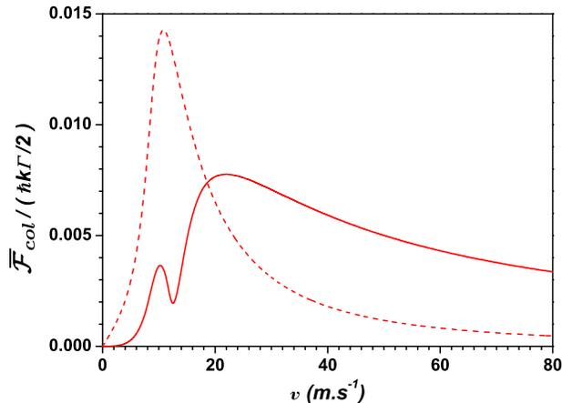
FIG. 7. (Color online) Mean value of the radiation-pressure-force transverse component ( $\overline{\mathcal{F}_{col}^{(t)}}$  - red solid line) vs atomic velocity in a SBM configuration. The mean value of the longitudinal component ( $\overline{\mathcal{F}_{col}^{(l)}}$  - red dashed line) has also been reported for reference. The calculations are performed for an optical detuning  $\Delta = -2\Gamma$  and a saturation parameter  $S_{col} = 0.1$ .
