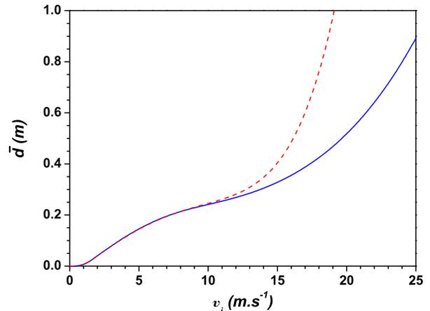
FIG. 8. (Color online) Mean distance needed for an atom with initial velocity  $v_i$  to be decelerated down to  $v_f = 1 \text{ m.s}^{-1}$ , when undergoing the radiation-pressure forces exerted in an ILC configuration (blue solid line) or in a SBM (red dashed line). The calculations are performed for an optical detuning  $\Delta = -2\Gamma$  and saturation parameters  $S_{col} = S_{iso} = 0.1$ .
