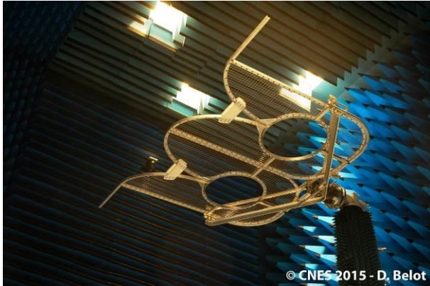
Figure 11. Photograph of the reference antenna during validation measurements
