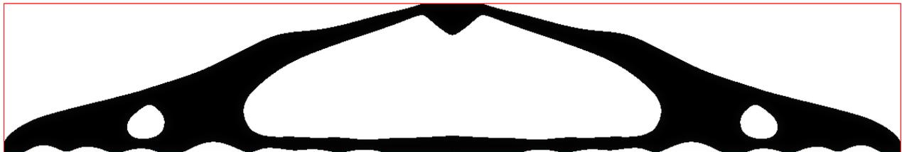
FIGURE 14. *Optimized two-dimensional MBB Beam for Problem (5.8), under both a geometric and perimeter constraint.*
