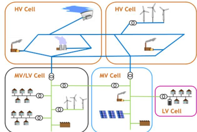
**Figure 2:** Schematic example of the proposed “Web-of-Cells” architecture
