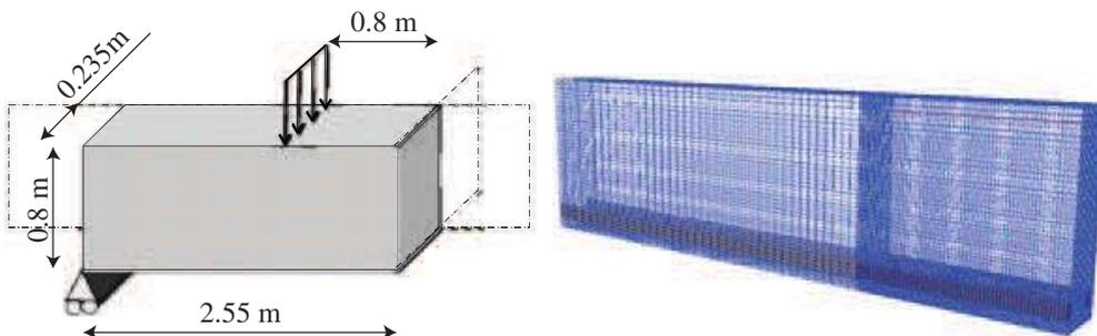
Figure 2. Mechanical scheme and mesh of a quarter of the reinforced concrete beam.
