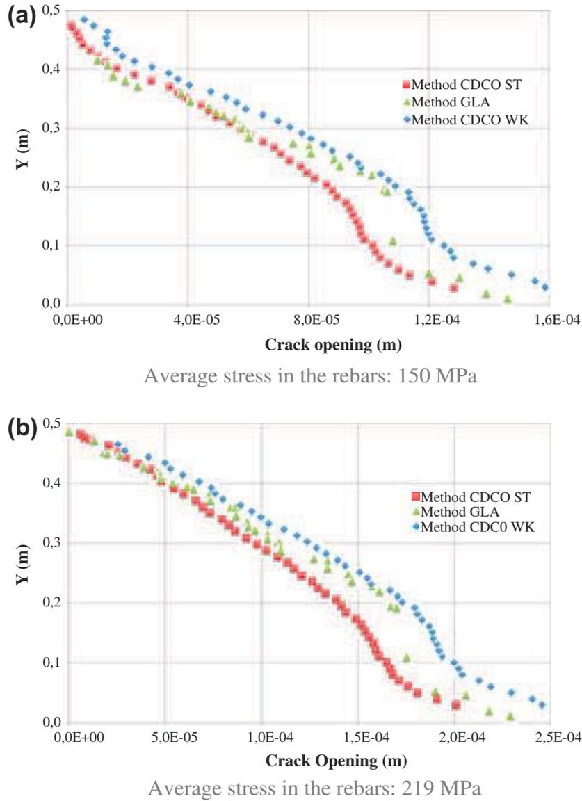
Figure 7. Evolution of crack opening along the height for a crack (at right in Figure 7) at the surface of the beam for two average stress levels in the lower rebars: 150 and 219 MPa during the loading of the stress profile along the bottom rebars.
