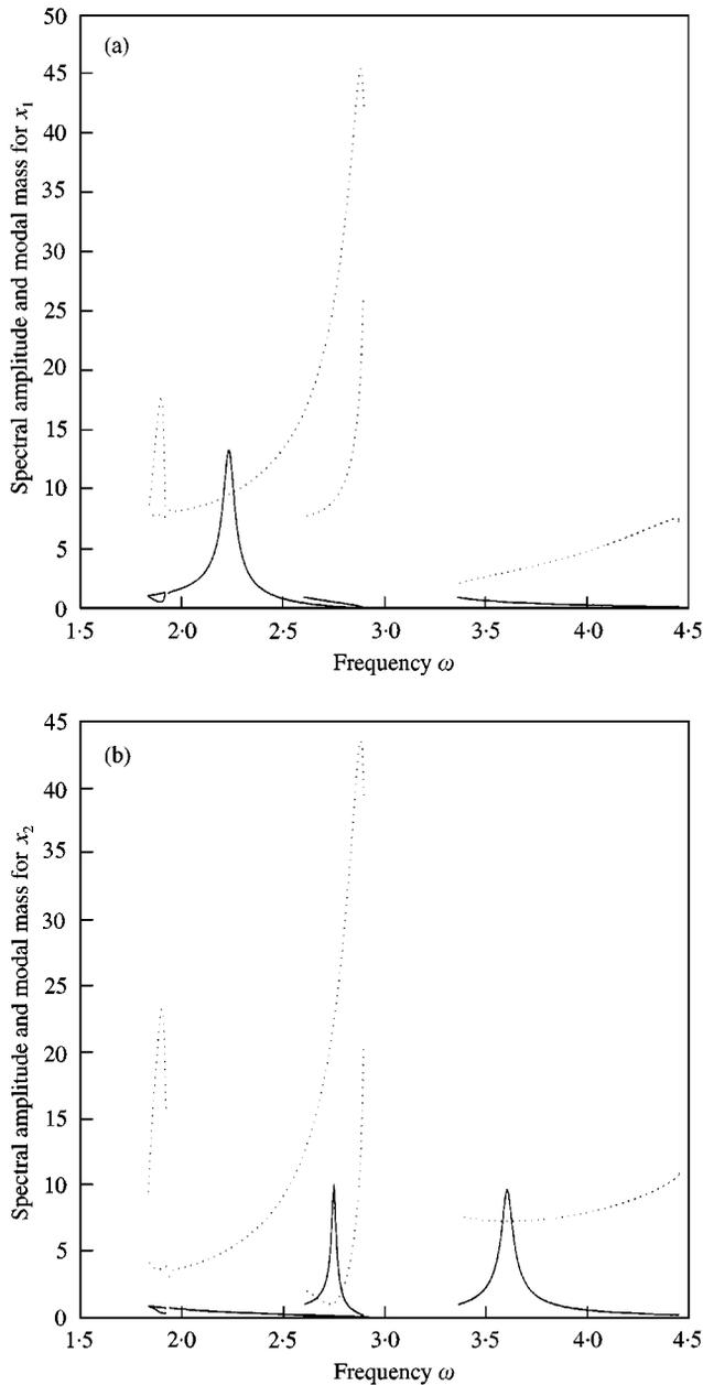
Figure 25. First-harmonic amplitude (dotted curve) and modal mass (solid curve) of the (1, 1)-periodic solutions: (a) first degree of freedom  $x_1$ ; (b) second degree of freedom  $x_2$ .
