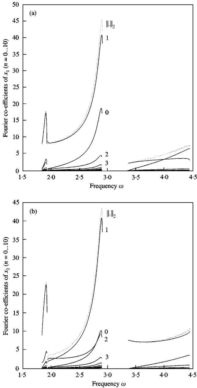
Figure 26. Fourier coefficients of the (1, 1)-periodic responses: (a) first degree of freedom  $x_1$ ; (b) second degree of freedom  $x_2$ .
