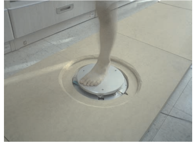
Figure 6. Installation of impact force sensor (PF-10, RION).
