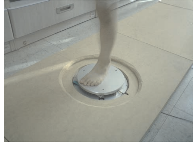
Figure 6. Installation of impact force sensor (PF-10, RION).
