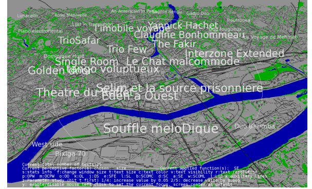
Figure 7: SE function result. After applying SE function, the NT is 29 and the OT is reduced to 7. It has the maximum RTS value, which is close to that of the original result.
