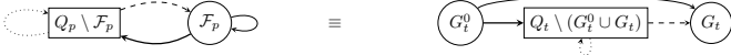
Fig. 1. Construction of \mathcal{A}_t from \mathcal{A}_p . Similar node shape represents equivalent state sets. Similar line style represents equivalent transition function between sets.
