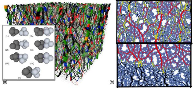
**Figure 4.** Snapshot of normal forces in (a) packing composed of non-convex particles (here  $\eta = 0.6$ ), and (b) packings composed of mixture of two shape for homogeneous (up) and segregated (down) packings. The forces are plotted in different colors depending on contact types. The inset shows contacts type for non-convex aggregate whereas in mixture we can distinguish disks-disks, discs-elongated and elongated-elongated contacts.
