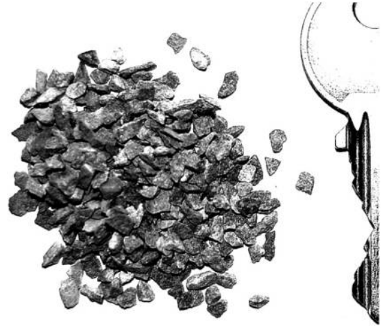
Fig. 2. 2 to 2.5 mm grains of shale quartzite sand from Trois Vallées.
