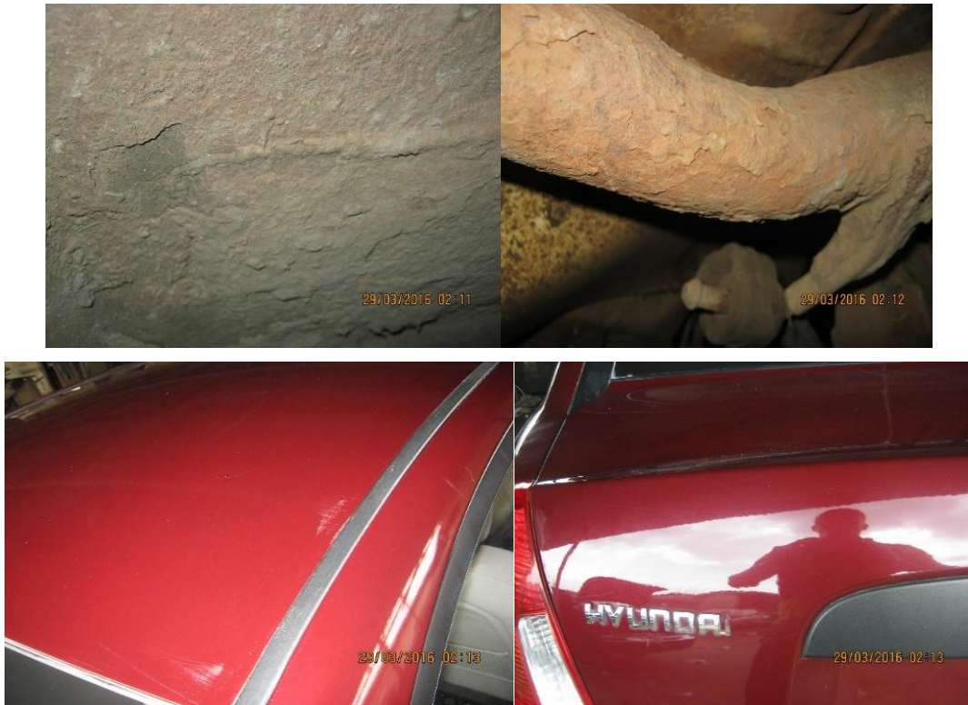
Fig. 30. Corrosion Effect on Different Parts of the Underneath of a Car (Manufacturer: HYUNDAI Model: Accent, Year of Manufacture: 2008).
