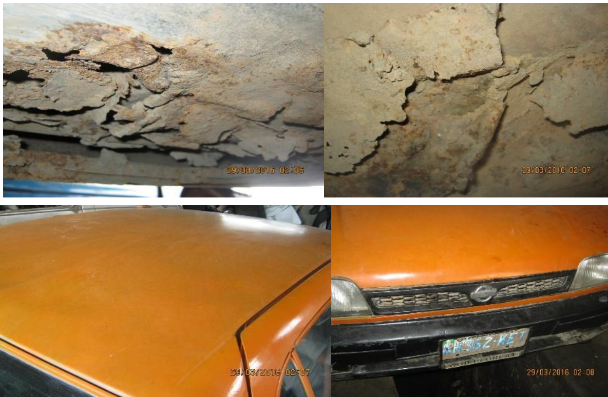
Fig. 9. Corrosion Effect on Different Parts of a Car Body (Manufacturer: NISSAN Model: Sunny 1.4L Year of Manufacture: 1991).
