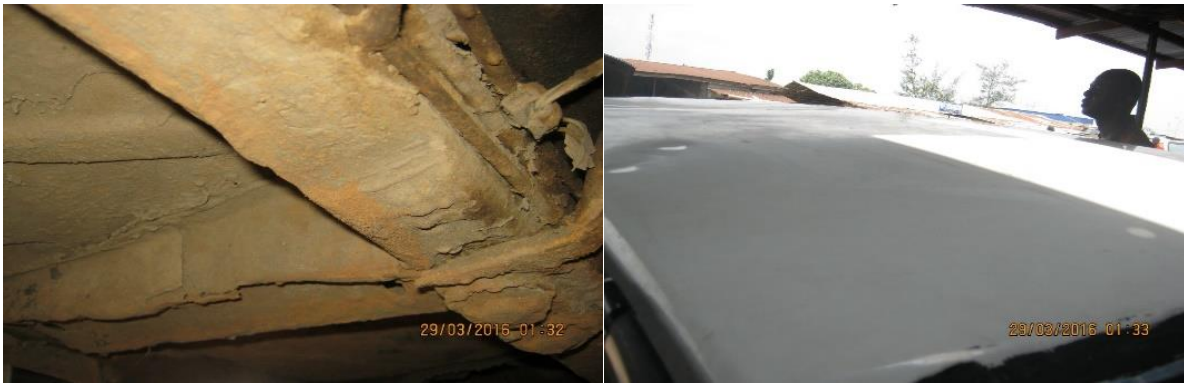
Fig. 8. Corrosion Effect on Different Parts of a Car Body (Manufacturer: VOLVO Model: 240GL, Year of Manufacture: 1987).
