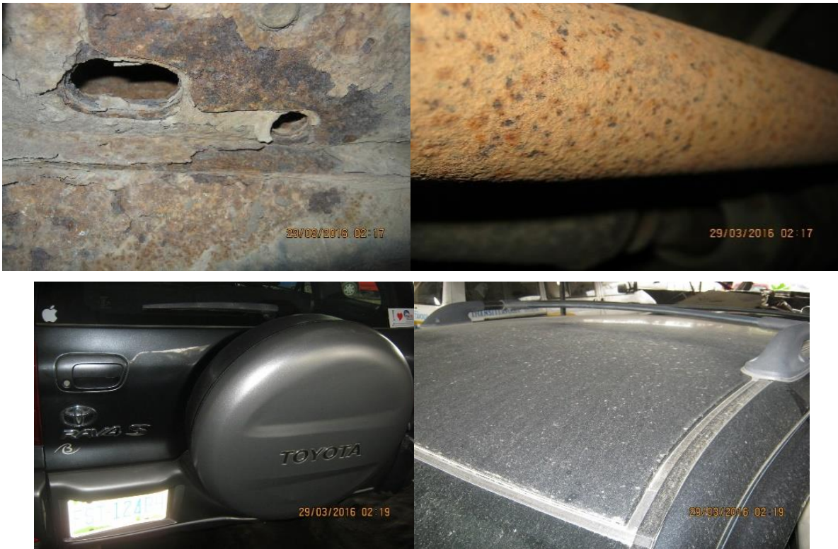
Fig. 26. Corrosion Effect on Different Parts of the Underneath of a Car (Manufacturer: TOYOTA Model: RAV4 S, Year of Manufacture: 2004).
