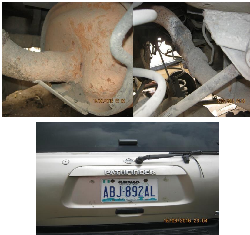
Fig. 27. Corrosion Effect on Different Parts of the Underneath of a Car (Manufacturer: NISSAN Model: Pathfinder, S.E 3.5, Year of Manufacture: 2005).
