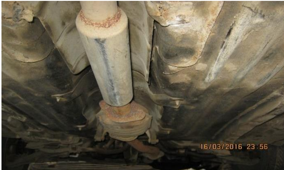
Fig. 1. Underneath Corrosion Effect on a Car in Uyo-Nigeria.
