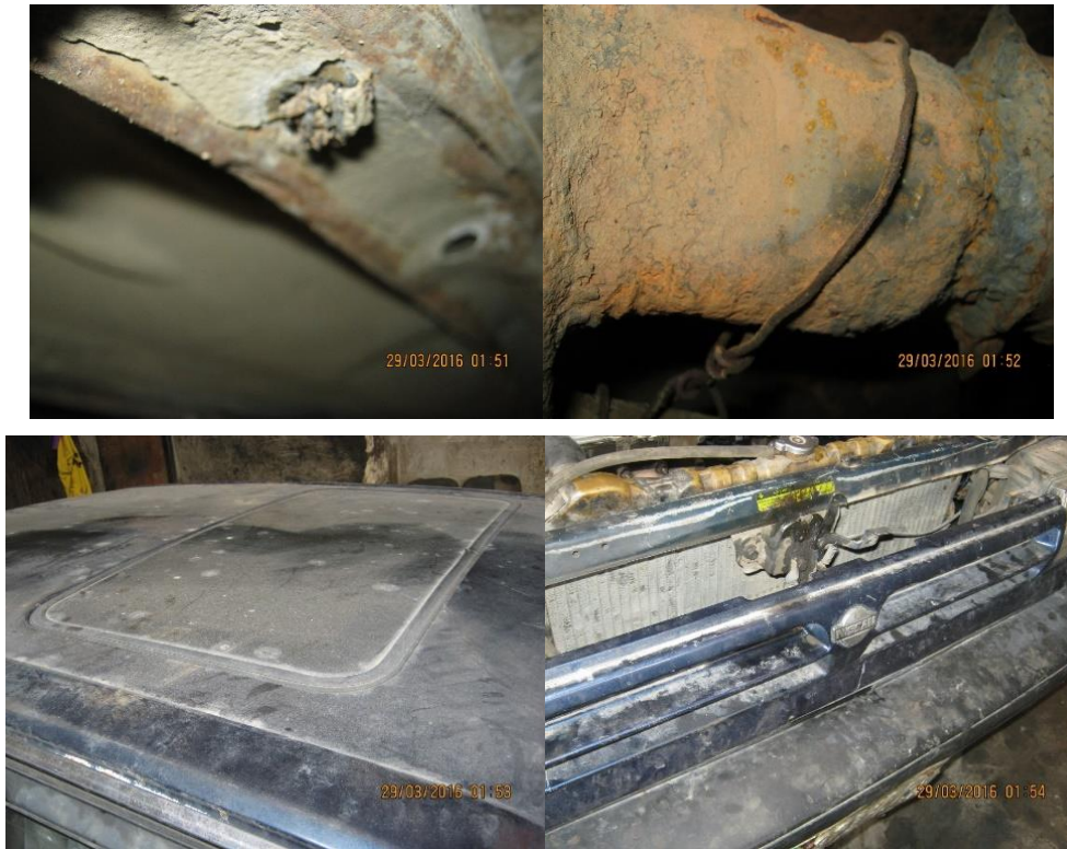
Fig. 14. Corrosion Effect on Different Parts of the Underneath of a Car (Manufacturer: NISSAN Model: Blue Bird, Year of Manufacture: 1998).
