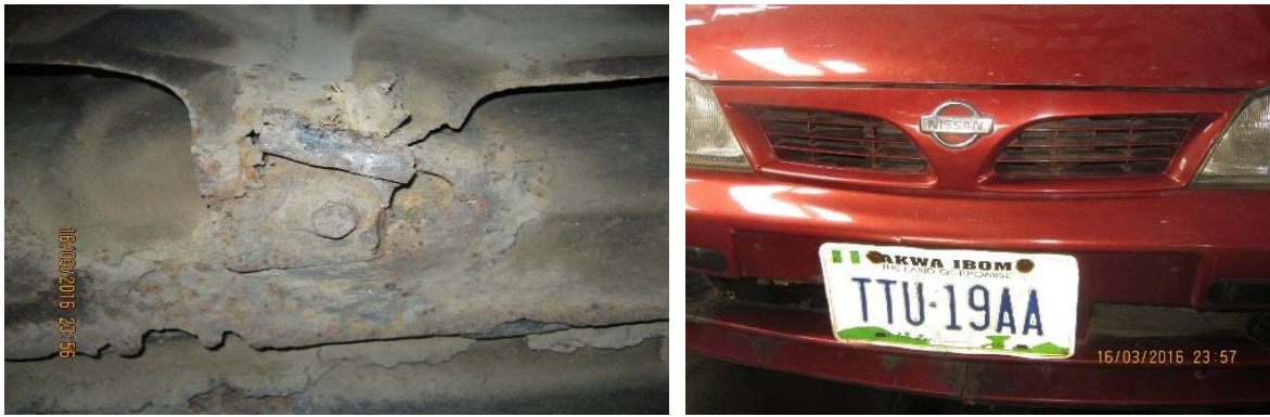
Fig. 12. Corrosion Effect on Different Parts of the Underneath of a Car (Manufacturer: NISSAN Model: Almera 1.6 SLX, Year of Manufacture: 1997).
