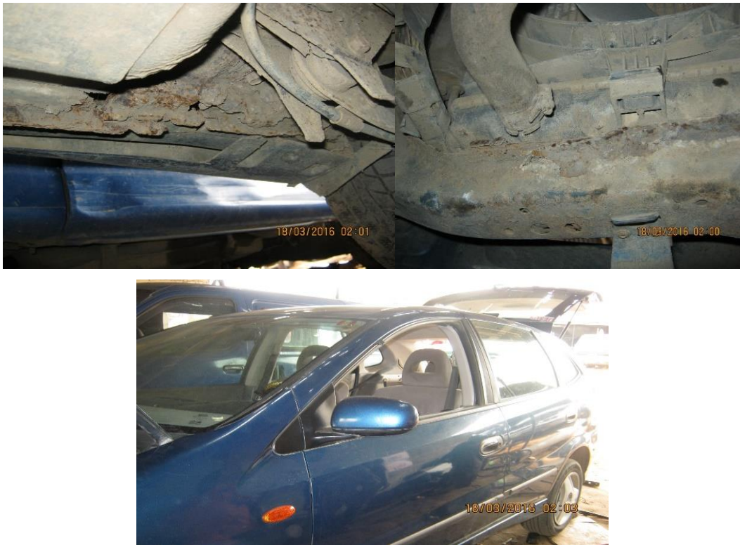
Fig. 18. Corrosion Effect on Different Parts of the Underneath of a Car (Manufacturer: NISSAN Model: Almera Tino, Year of Manufacture: 2001).
