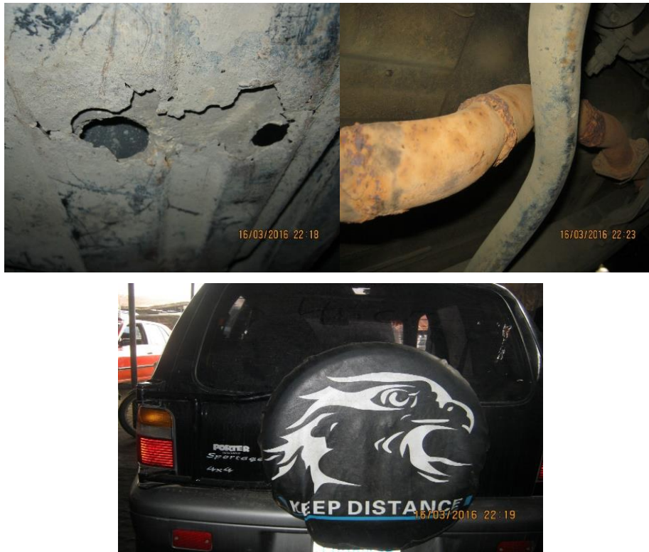
Fig. 28. Corrosion Effect on Different Parts of the Underneath of a Car (Manufacturer: KIA Model: Porter, Year of Manufacture: 2008).
