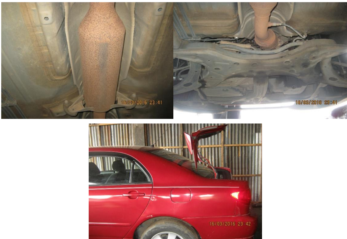
Fig. 25. Corrosion Effect on Different Parts of the Underneath of a Car (Manufacturer: TOYOTA Model: Corolla S Year of Manufacture: 2003).
