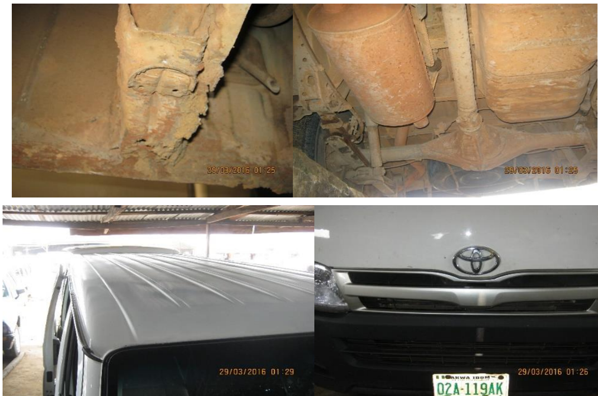
Fig. 31. Corrosion Effect on Different Parts of the Underneath of a Car (Manufacturer: TOYOTA Model: Haice bus, Year of Manufacture: 2009).
