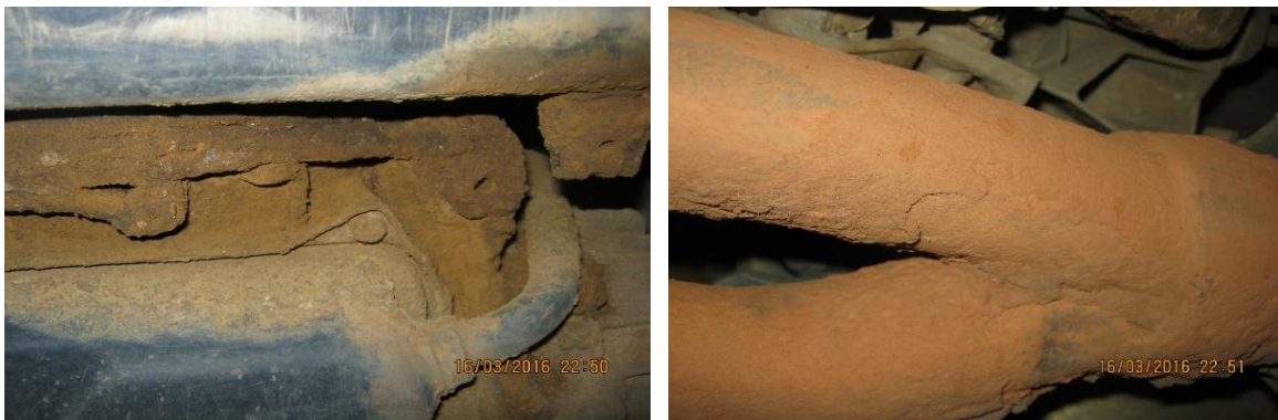
Fig. 9. Corrosion Effect on Different Parts of a Car Body (Manufacturer: NISSAN Model: Sunny 1.4L Year of Manufacture: 1991).
