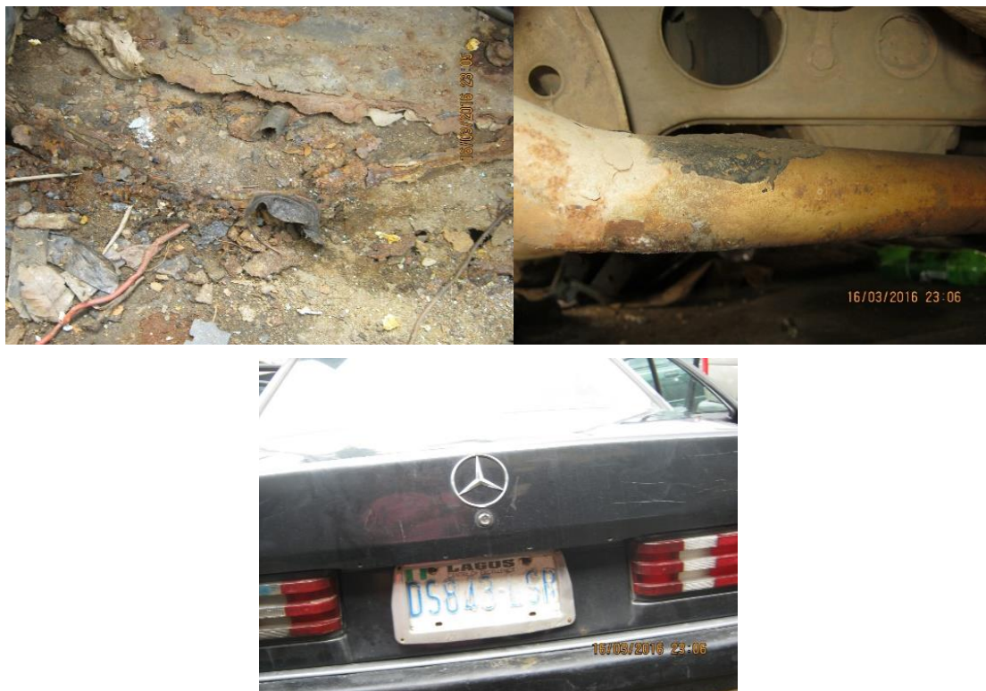
Fig. 21. Corrosion Effect on Different Parts of the Underneath of a Car (Manufacturer: Mercedes-Benz Model: BENZ 190, Year of Manufacture: 2002).
