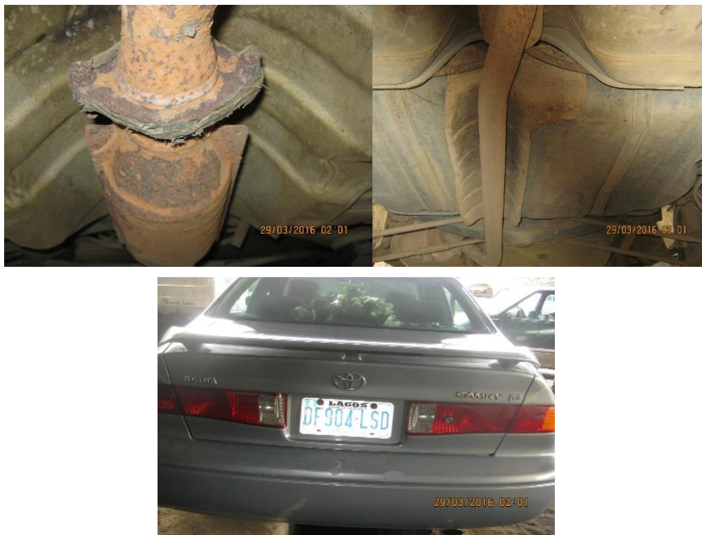
Fig. 17. Corrosion Effect on Different Parts of the Underneath of a Car (Manufacturer: TOYOTA Model: Camry LE, Year of Manufacture: 1999).
