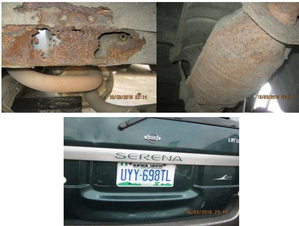
Fig. 23. Corrosion Effect on Different Parts of the Underneath of a Car (Manufacturer: NISSAN Model: Serena LMT 200, Year of Manufacture: 2002).
