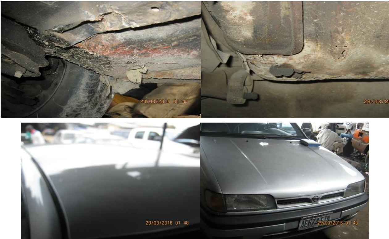
Fig. 24. Corrosion Effect on Different Parts of the Underneath of a Car (Manufacturer: NISSAN Model: Sunny 1.6SLX, Year of Manufacture: 2002).
