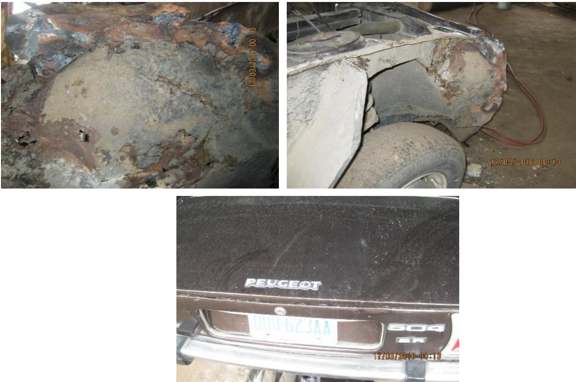
Fig. 3. Corrosion Effect on Different Parts of a Car Body (Manufacturer: Peugeot, Model: 504 SR Year of Manufacture: 1985).
