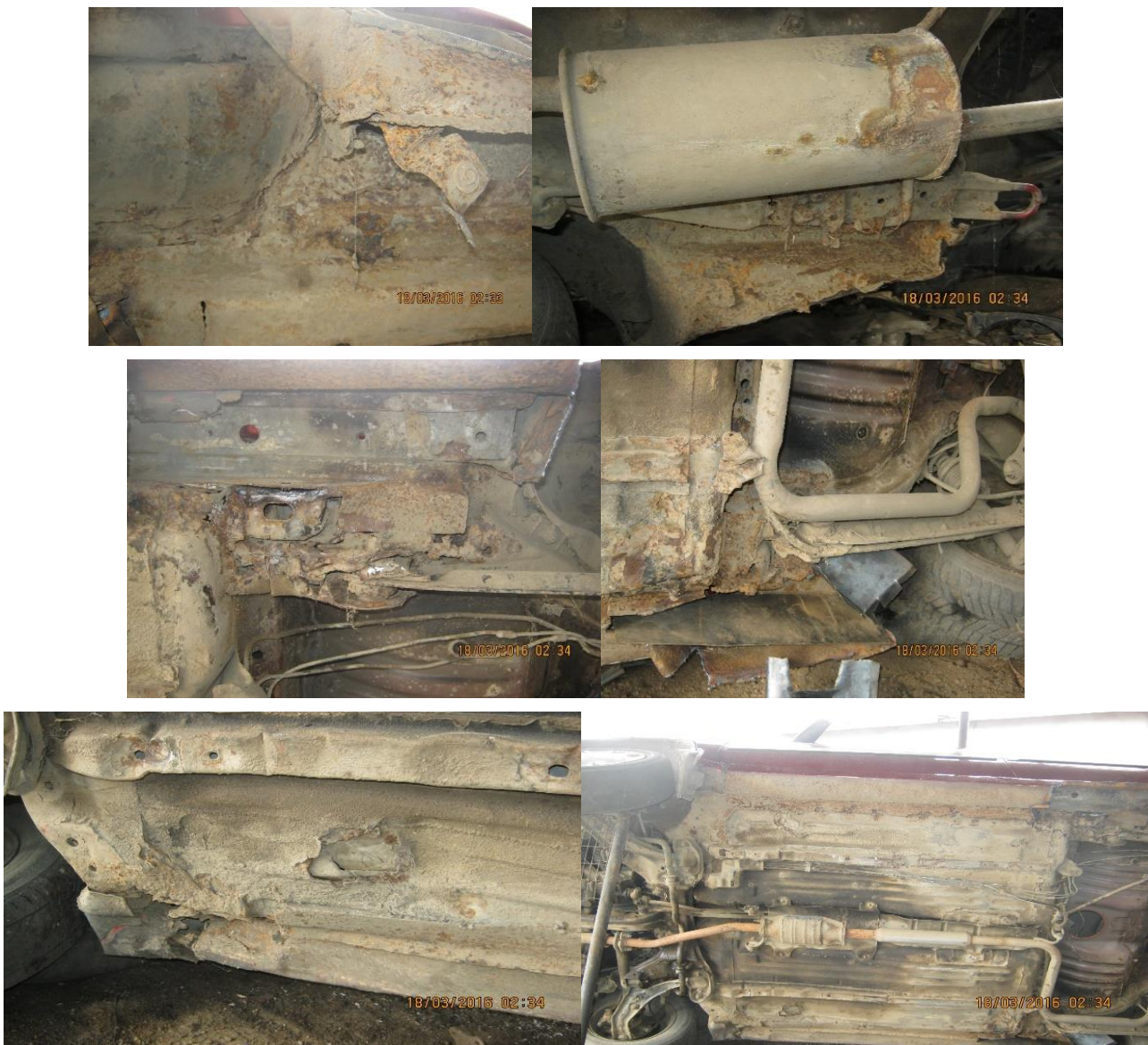
Fig. 13. Corrosion Effect on Different Parts of the Underneath of a Car (Manufacturer: NISSAN Model: Almera 1.6 SLX, Year of Manufacture: 1997).
