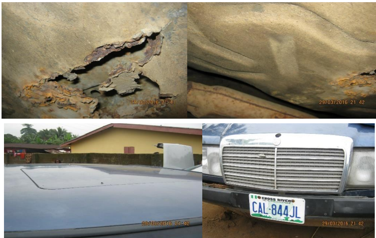
Fig. 6. Corrosion Effect on Different Parts of a Car Body (Manufacturer: Mercedes-Benz, Model: V booth 300 E, Year of Manufacture: 1985).
