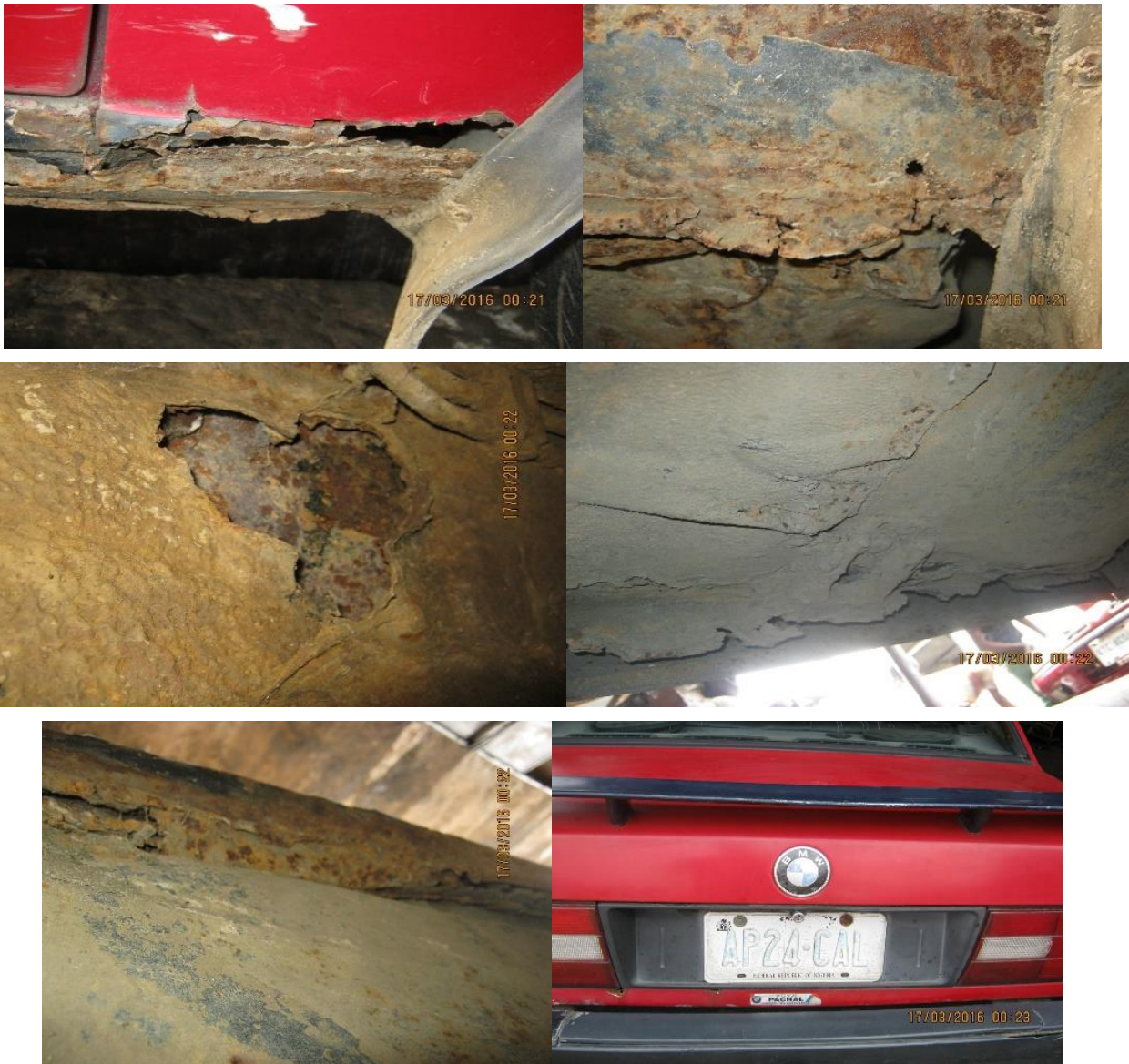
Fig. 7. Corrosion Effect on Different Parts of a Car Body (Manufacturer: BMW Model: E 30, Year of Manufacture: 1987).
