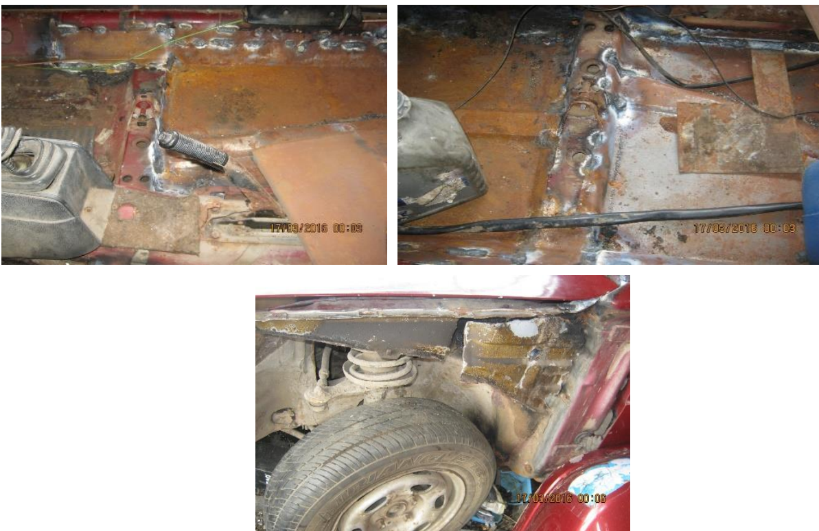
Fig. 4 Corrosion Effect on Different Parts of a Car Body (Manufacturer: Volkswagen Model: Passat 402, Year of Manufacture: 1985)
