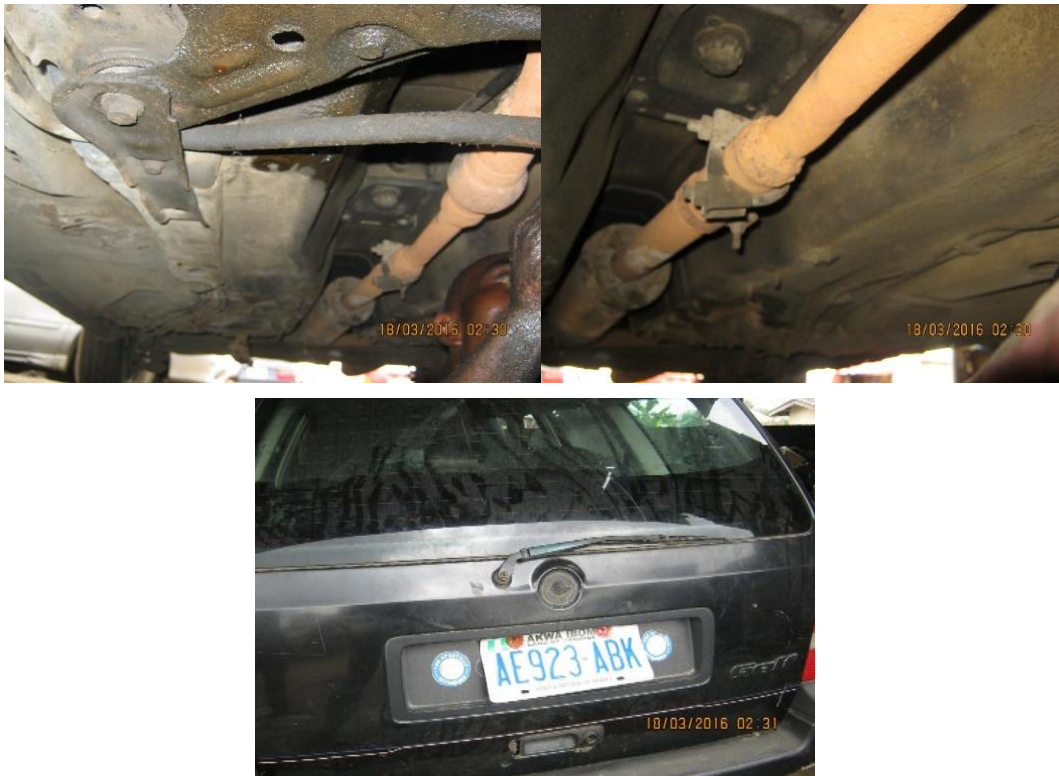
Fig. 20. Corrosion Effect on Different Parts of the Underneath of a Car (Manufacturer: Volkswagen Model: GOLF 3.0 Wagon, Year of Manufacture: 2001).
