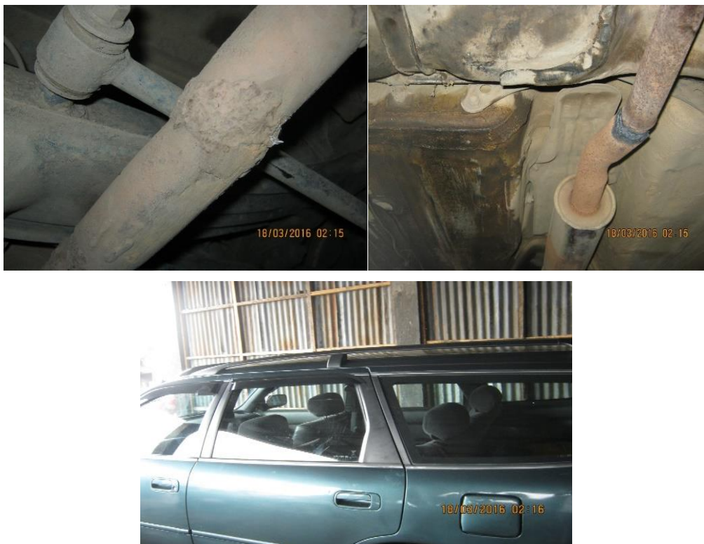
Fig. 19. Corrosion Effect on Different Parts of the Underneath of a Car (Manufacturer: TOYOTA Model: Camry 2.2 XL, Year of Manufacture: 2001).
