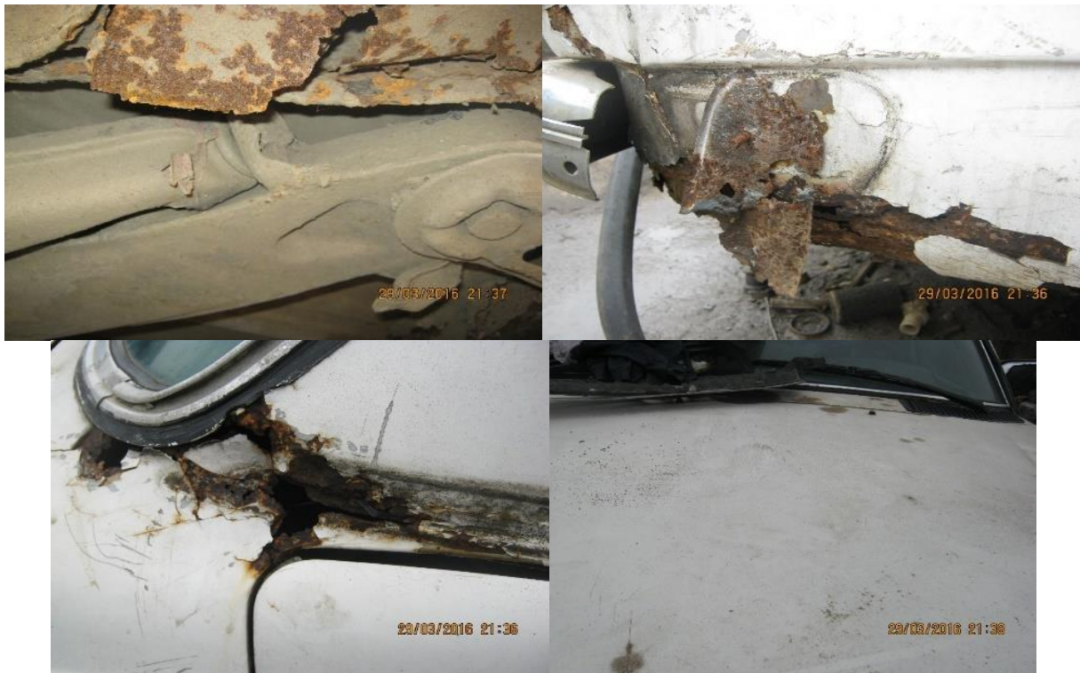
Fig. 2. Corrosion Effect on different parts of a car body (Manufacturer: Mercedes-Benz Model: Flat booth 200 E, Year of Manufacture: 1975).
