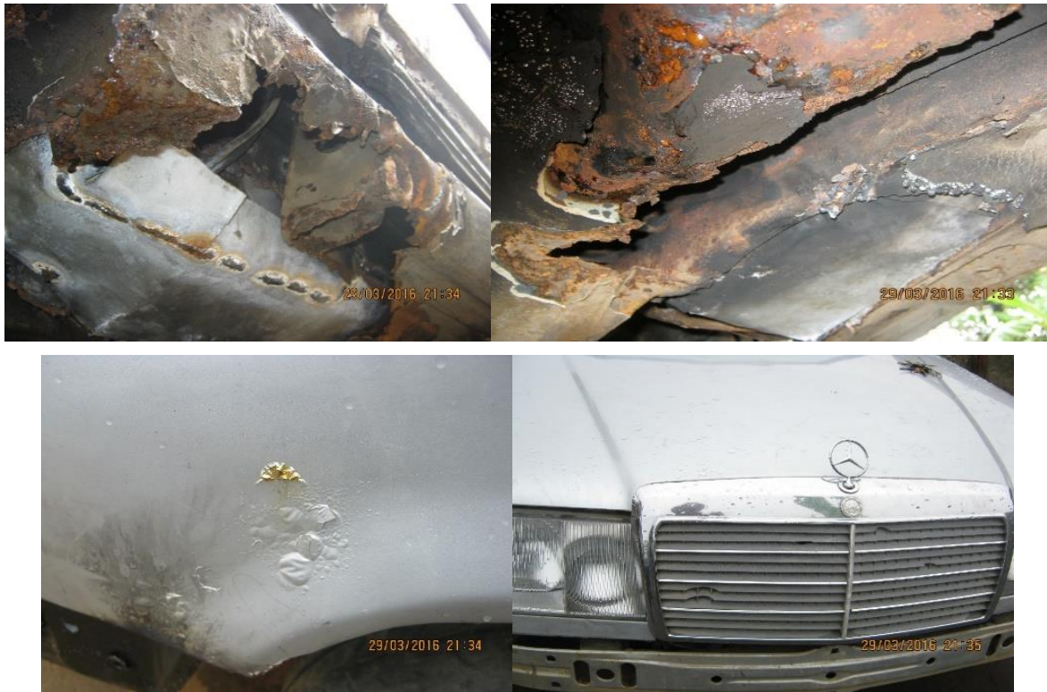
Fig. 5. Corrosion Effect on Different Parts of a Car Body (Manufacturer: Mercedes-Benz Model: V booth 230 E, Year of Manufacture: 1985).
