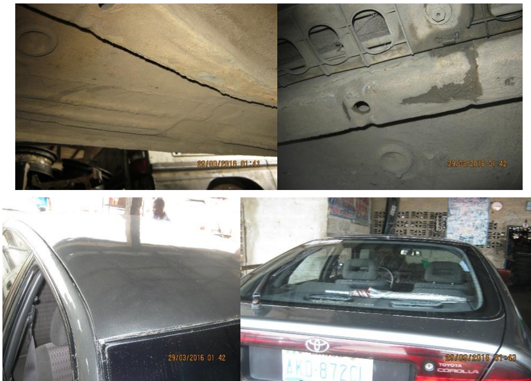
Fig. 15. Corrosion Effect on Different Parts of the Underneath of a Car (Manufacturer: TOYOTA Model: Corolla, Year of Manufacture: 1998).
