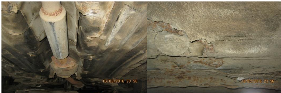
Fig. 11. Corrosion Effect on Different Parts of the Underneath of a Car (Manufacturer: TOYOTA Model: Camry 2.2 GL, Year of Manufacture: 1996).
