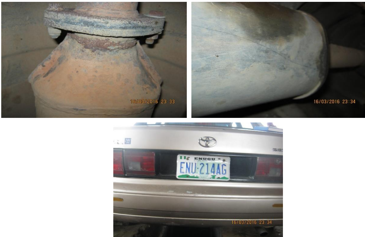
Fig. 11. Corrosion Effect on Different Parts of the Underneath of a Car (Manufacturer: TOYOTA Model: Camry 2.2 GL, Year of Manufacture: 1996).
