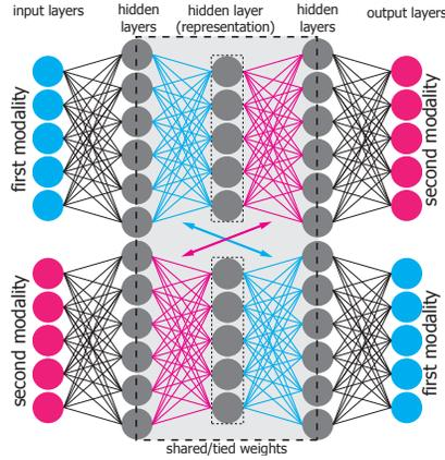
**Fig. 1.** Architecture of bidirectional symmetrical deep neural networks
