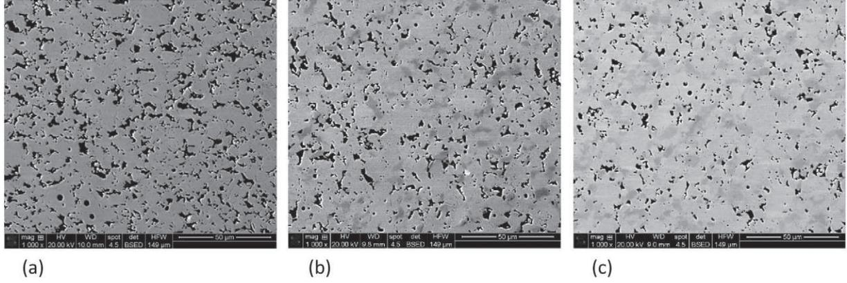
Fig. 3. SEM images of the specimen surfaces for pure YSZ matrix (a), YSZ and 10 vol.% MoSi<sub>2</sub> (b) and YSZ with 20 vol.% MoSi<sub>2</sub> (c).
