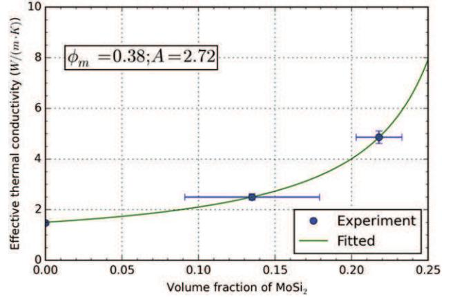
Fig. 8. Thermal conductivity of composites consisting of MoSi<sub>2</sub> spheres in an YSZ matrix. The solid line reflects theoretical predictions using Eqs. (3)–(6). Dots show experimental values measured at room temperature for actual volume fraction of MoSi<sub>2</sub> particles, as stated in Table 1.
