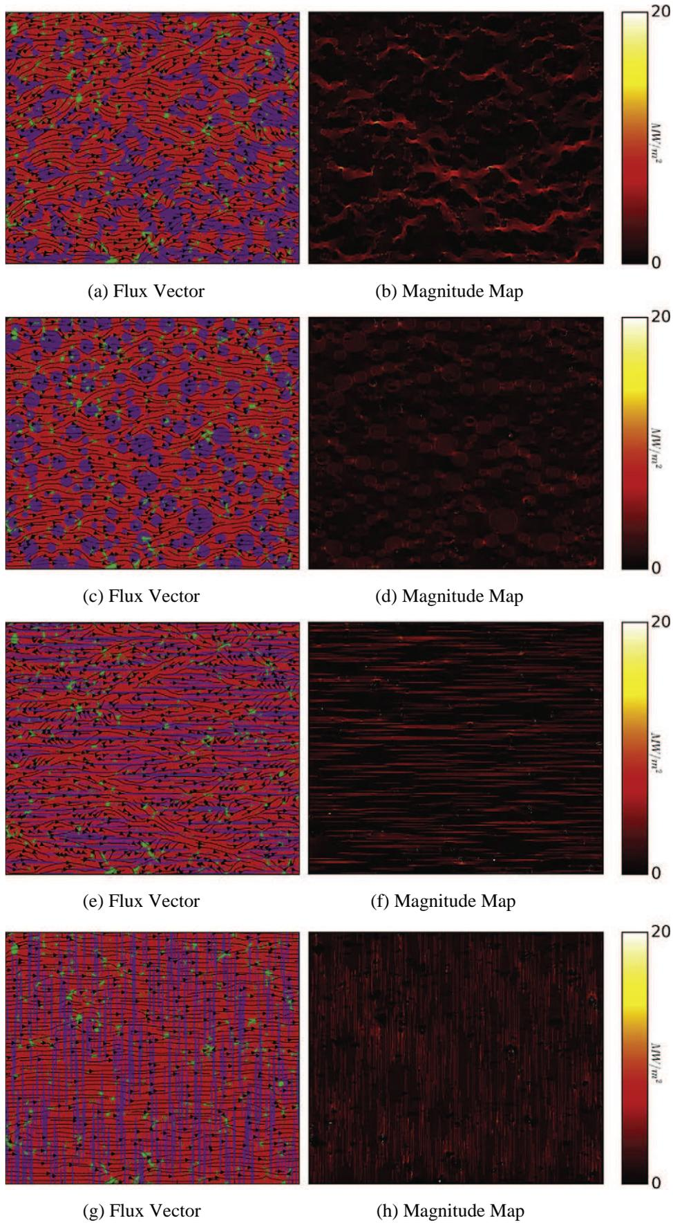
**Fig. 12.** Heat fluxes inside the ceramic composites with different MoSi<sub>2</sub> shapes: real microstructure,  $k_{eff} = 4.18 \text{ Wm}^{-1} \text{ K}^{-1}$  (a-b);  $a:c = 1:1$ ,  $k_{eff} = 3.38 \text{ Wm}^{-1} \text{ K}^{-1}$  (c-d);  $a:c = 32:1$ ,  $k_{eff} = 7.77 \text{ Wm}^{-1} \text{ K}^{-1}$  (e-f) and  $a:c = 1:32$ ,  $k_{eff} = 2.75 \text{ Wm}^{-1} \text{ K}^{-1}$  (g-h). The shape of MoSi<sub>2</sub> strongly affects the heat fluxes as they serve as channels for thermal flow.
