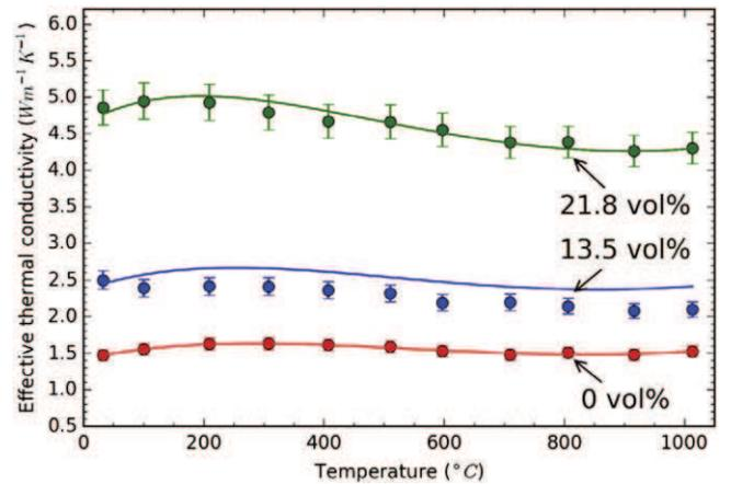
Fig. 9. Thermal conductivity of composites consisting of MoSi<sub>2</sub> spheres in an YSZ matrix. Dots show experimental data fitted into the Nielsen model (solid line) according to the actual volume fraction of MoSi<sub>2</sub> particles [26].
