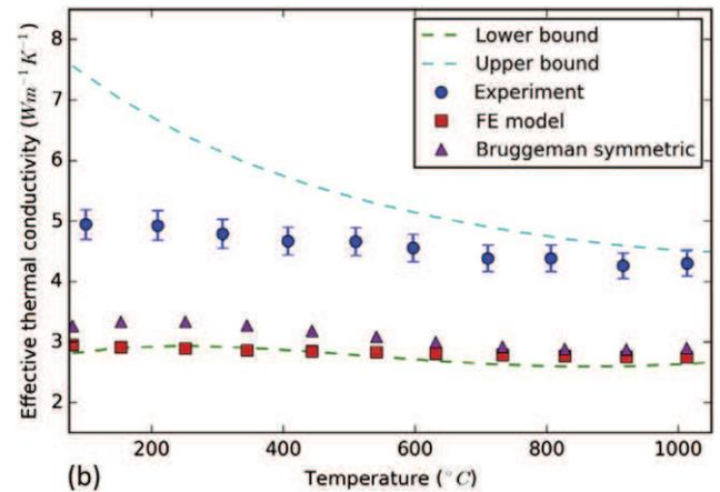
Fig. 7. Comparison of the temperature dependent thermal conductivity based on FE and the Bruggeman model solution for composite samples with 10 vol.% (a) and 20 vol.% MoSi<sub>2</sub> filler (b). Dashed lines show lower and upper boundary regions for the asymmetric Bruggeman model.
