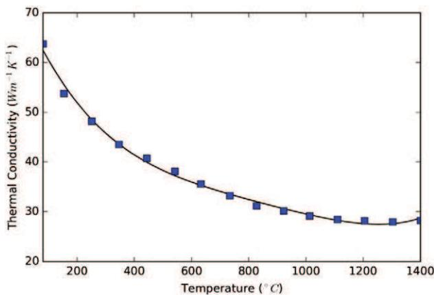
**Fig. 2.** Thermal conductivity of MoSi<sub>2</sub> as a function of temperature [11].
