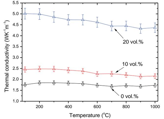
Fig. 6. Thermal conductivity of the YSZ/MoSi<sub>2</sub> as a function of temperature calculated using Eq. (1).
