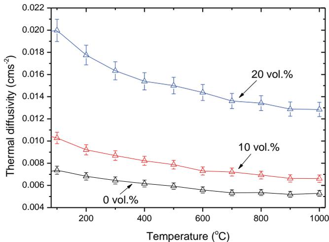
Fig. 5. Thermal diffusivity of the YSZ/MoSi<sub>2</sub> as a function of temperature.
