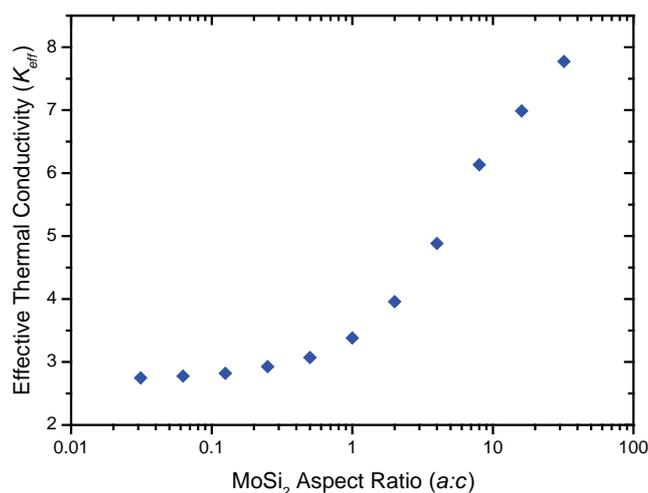
**Fig. 11.** Effective thermal conductivity values as a function of the  $\text{MoSi}_2$  aspect ratio  $a:c$  calculated for modelled artificial microstructures.
