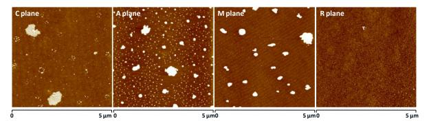
**Figure 1**: Representative AFM images (5 x 5 μm<sup>2</sup>, Peak Force Tapping mode, z-scale 4 nm) of planar  $Mo/\alpha$ -Al<sub>2</sub>O<sub>3</sub> model catalysts with a Mo surface loading of 3.5 at.nm<sup>-2</sup> after impregnation and calcination at 450 °C for 2 h for various alumina orientations: C (0001), A (11 $\overline{2}$ 0), M (10 $\overline{1}$ 0) and R (1 $\overline{1}$ 02) planes.
