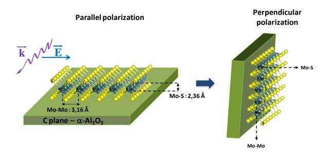
**Scheme 2**: Basal orientation of MoS<sub>2</sub> slabs on the C (0001) plane of  $\alpha$ -Al<sub>2</sub>O<sub>3</sub> and change of polarization with respect to the synchrotron beam: parallel on the left and perpendicular on the right.  $\vec{k}$  is the wave vector and  $\vec{E}$  is the electric field vector.
