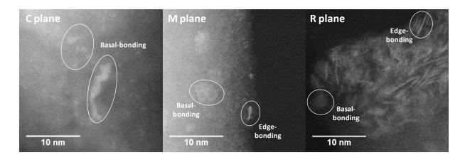
**Figure 11**: Typical HR HAADF-STEM images of sulfided model Mo/ $\alpha$ -Al<sub>2</sub>O<sub>3</sub> catalysts (Mo surface loading is 3.5 at.nm<sup>-2</sup>) supported on the C (0001), M (10 $\overline{10}$ ) and R (1 $\overline{10}$ 2) orientations of  $\alpha$ -Al<sub>2</sub>O<sub>3</sub>. Samples were prepared by Mo impregnation, calcination at 450°C for 2h and sulfidation at 300°C under H<sub>2</sub>S/H<sub>2</sub>.
