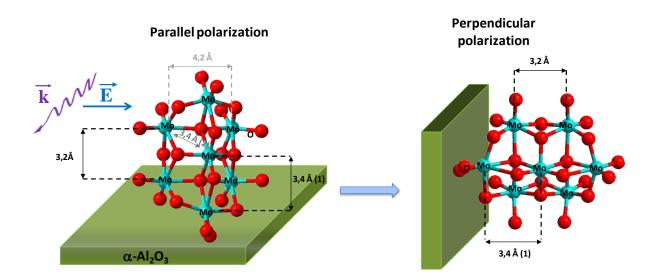
**Scheme 1**: "Edge-on" orientation of an heptamolybdate-like species on the R ( $1\overline{1}02$ ) plane of  $\alpha$ -Al<sub>2</sub>O<sub>3</sub>.  $\vec{k}$  is the wave vector and  $\vec{E}$  is the electric field vector of the synchrotron beam. Parallel and perpendicular polarizations refer to the orientation of  $\vec{E}$  with respect to the surface of the wafer.
