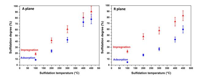
**Figure 12**: Comparison of sulfidation degree as a function of sulfidation temperature for model  $Mo/\alpha$ - $Al_2O_3$  catalysts prepared by impregnation (red triangles) and by equilibrium adsorption (blue circles) on the A (11 $\overline{2}0$ ) plane (Mo loading of 3.5 at.nm<sup>-2</sup>) and on the R (1 $\overline{1}02$ ) plane (Mo loading of 1.0 at.nm<sup>-2</sup>).
