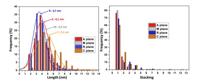
**Figure 8**: MoS<sub>2</sub> size and stacking distribution for model Mo/ $\alpha$ -Al<sub>2</sub>O<sub>3</sub>catalysts supported on C (0001), R (1 $\overline{10}$ 2), A (11 $\overline{20}$ ) and M (10 $\overline{10}$ 0) planes sulfided at 300°C in H<sub>2</sub>S/H<sub>2</sub> (Mo surface loading is 3.5 at.nm<sup>2</sup>).
