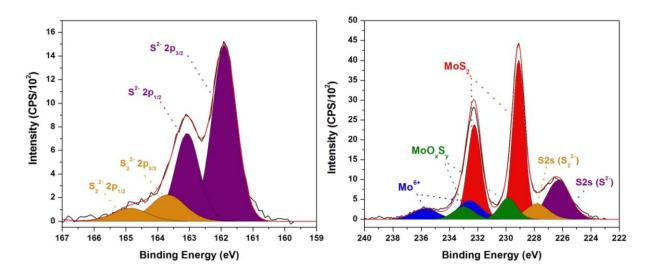
**Figure 4**: Decomposition of S2p, Mo3d and S2s XPS peaks for a model Mo/ $\alpha$ -Al<sub>2</sub>O<sub>3</sub> catalyst supported on the M (1010) plane (3.5 atMo/nm<sup>2</sup>) and sulfided at 450 °C for 2 h.
