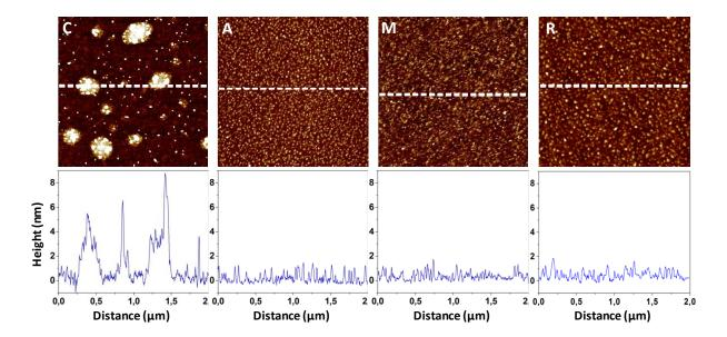
**Figure 6**: Representative AFM images  $(2.0 \times 2.0 \ \mu\text{m}^2)$ , peak force tapping mode in air, z-scale 8.0 nm) obtained on model Mo/ $\alpha$ -Al<sub>2</sub>O<sub>3</sub> catalysts supported on C (0001), R (1102), A (1120) and M (1010) planes and sulfided at 450 °C (Mo surface loading is 3.5 at.nm<sup>-2</sup>). Cross sections were taken at the position indicated by the white dashed lines on the images.
