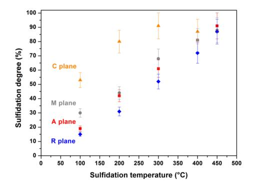
**Figure 5**: Sulfidation degree for model Mo/ $\alpha$ -Al<sub>2</sub>O<sub>3</sub> catalysts supported on C (0001), A (11 $\overline{2}$ 0), M (10 $\overline{1}$ 0) and R (1 $\overline{1}$ 02) planes as a function of sulfidation temperature with a Mo surface loading of 3.5 at.nm<sup>-2</sup>.
