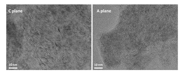
**Figure 7**: Typical TEM images of model Mo/ $\alpha$ -Al<sub>2</sub>O<sub>3</sub> catalysts supported on A (11 $\overline{2}$ 0) and C (0001) planes sulfided at 300°C in H<sub>2</sub>S/H<sub>2</sub> (Mo surface loading is 3.5 at.nm<sup>-2</sup>).
