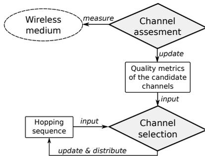
Figure 1: Overview of the adaptive channel selection process [4].
