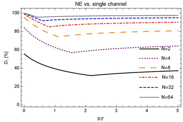
Fig. 4. Relative utility gain between the NE vs. single channel SKG:  $D_1 = (u^{NE} - u^{single})/u^{NE}$  as a function of  $P/\Gamma$  for  $\Gamma = \sigma_H^2 = \sigma_A^2 = \sigma_B^2 = 1$  and  $N \in \{2, 4, 8, 16, 32, 64\}$ .
