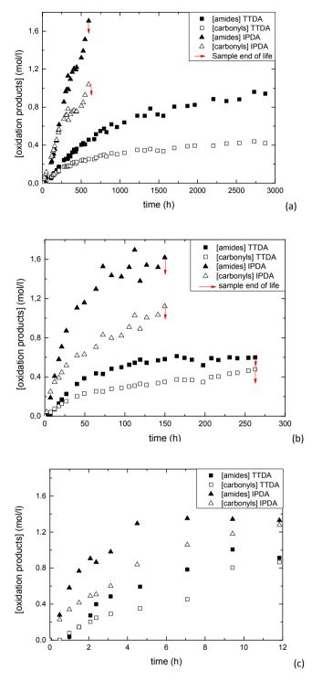
Fig. 3. Changes in concentration of amides and carbonyls under air at 110  $^{\circ}$ C (a), 150  $^{\circ}$ C (b) and 200  $^{\circ}$ C (c).
