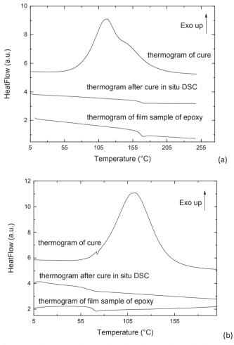
Fig. 12. DSC thermogram of DGEBA/IPDA (a) and DGEBA/ITDA (b) of uneacted expoy + diamine mixture and comparison of thermogram for epoxy cured in situ in the DSC cell and cured according to the procedure detailed in "EXPERIMENTAL SECTION".
