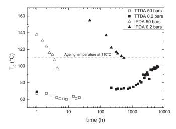
Fig. 8. Glass transition temperature  $(T_g)$  changes as a function of time for at 110  $^\circ\text{C}$  under 0.2 and 50 bars oxygen.
