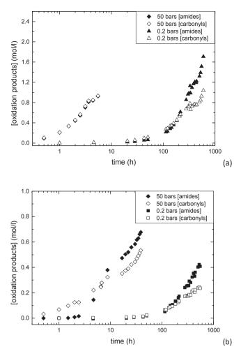
Fig. 6. Amides and carbonyls build up for DGEBA/IPDA (a) and DGEBA/TTDA (b) at 110  $^\circ\text{C}$  under 0.2 bars (empty symbol) and under 50 bars (full symbol) of oxygen.
