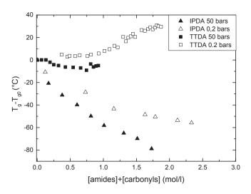
**Fig. 9.**  $T_g-T_{g0}$  with  $T_{g0}$  being initial glass transition temperature, as a function of sum of amides and carbonyls concentration for DGEBA/IPDA and DGEBA/IPDA at 110 °C under 0.2 bars (empty symbol) and 50 bars of oxygen (full symbol).
