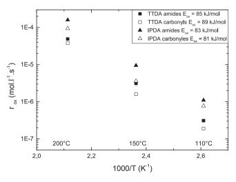
Fig. 4. Arrhenius plot of oxidation rate for DGEBA/IPDA and DGEBA/TTDA under air and activation energies of oxidation ( $E_{\rm ox}$ ).
