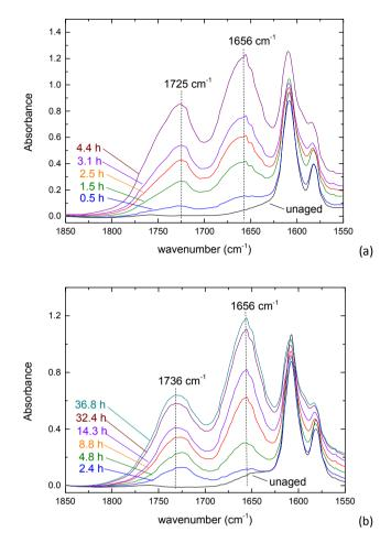
Fig. 5. FTIR spectra of DGEBA/IPDA (a) and DGEBA/TTDA (b) during oxidative thermal ageing at 110  $^\circ C$  under 50 bars of oxygen.
