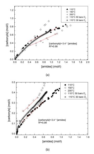
**Fig. 7.** Correlation between oxidation products formation for (a) DGEBA/IPDA and (b) DGEBA/TTDA.
