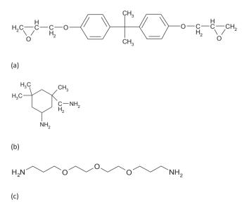
**Fig. 1.** Chemical structure of (a) bisphenol A diglycidyl ether (DGEBA), (b) isophorone diamine (IPDA) (c) 4,7,10-Trioxa-1,13-tridecanediamine (TTDA).
