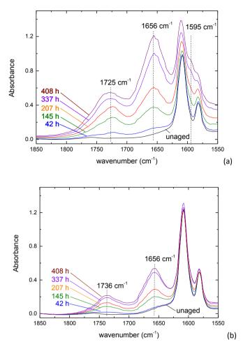
Fig. 2. FTIR spectra of DGEBA/IPDA (a) and DGEBA/TTDA (b) during oxidative thermal ageing at 110  $^\circ\text{C}.$
