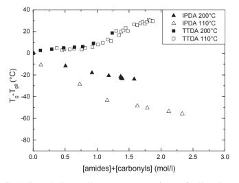
**Fig. 10.** Changes in glass transition temperature versus the sum of amides and carbonyls concentration for DGEBA/IPDA and DGEBA/TTDA in air at 110 °C at 110 °C (empty symbol) and 200 °C (full symbol).
