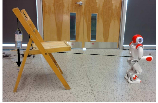
Fig. 5. Experimental setup used to apply a known external force
