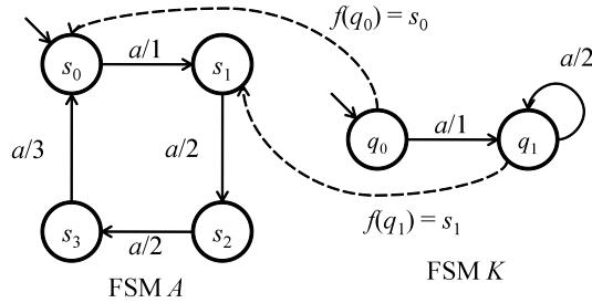
Figure 2: Initial  $Z$ -quotient of FSM  $A$
