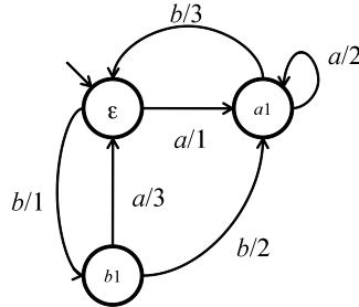
Figure 6: Initial  $\{a\}$ -Quotient  $K$  of FSM  $A$
