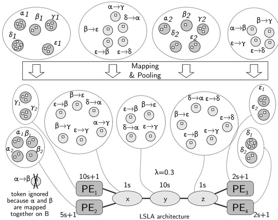
Figure 9: Computing the cost of executing the BSP model in Figure 8 on an LSLA architecture. The obtained cost is  $31 + 31 + 11 + 11 + 11 + 6 + 0.3 (6 + 40 + 6) + 7 + 5 + 11 + 5 = 144.6 \nu$  (Equation 4).
