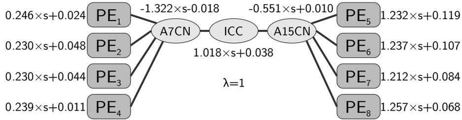
Figure 14: LSLA dynamic energy model inferred from energy measurements with computational quanta in ns, communication quanta in Bytes, and energy data vector  $d$  in nJ.  $PE_{1-4}$  are Cortex-A7 cores and  $PE_{5-8}$  are Cortex-A15 cores.
