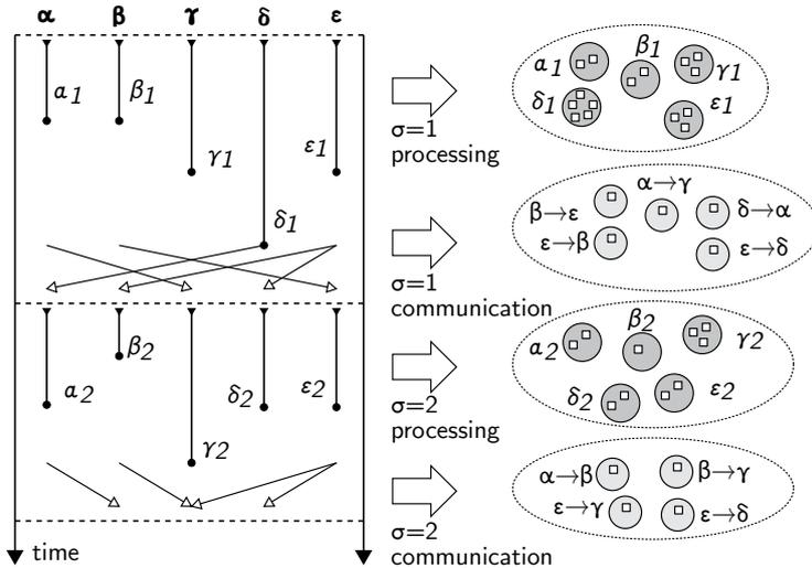
Figure 8: Extracting the activity of a BSP model.
