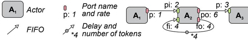
Figure 2: Example of an SDF Graph.
