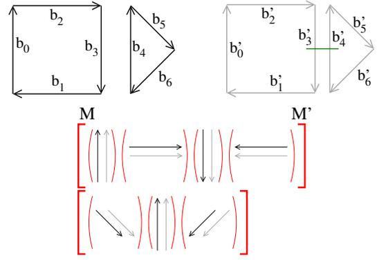
Figure 4: Example of two EBM-LCC comparison:  $M_1$  is composed with a square and a triangle which are not adjacent, while  $M_2$  has also one square and one triangle but adjacent (thus only one connected component).  $M_1$  darts are drawn in black, while  $M_2$  darts are drawn in gray.
