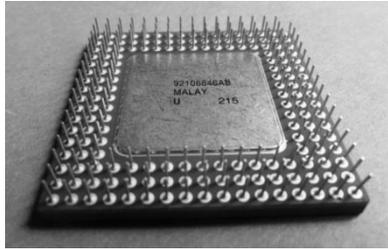
**Figure 5c:** Intel 80486 in 168-pin PGA (underside)
