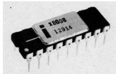
**Figure 5a:** Intel 8008 in 18-pin dual-in-line package
