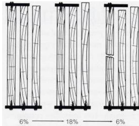
**Figure 6:** Evidence of compression set according to Hoadley (1995).
