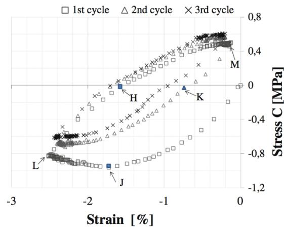
**Figure 7:** Stress of fully restrained specimen versus the unloaded strain of a specimen subjected to the same wetting-drying cycles (25°C, 30-80-30%RH): (square) 1st cycle, (triangle) 2nd cycle, (x) 3rd cycle. OH: compression set; OK dimensional loss for restrained or partially restrained specimens. J: stress peak, L: end of 1st adsorption; M: end of 1st cycle and start of 2nd (Mazzanti et al 2015)
