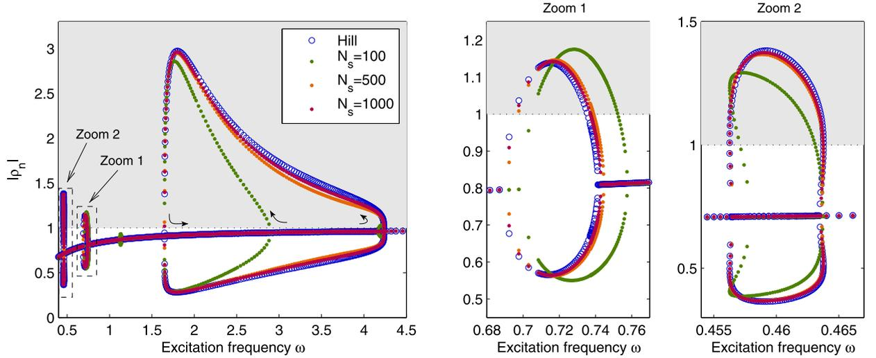
**Fig. 2.** The  $N = 2$  Floquet multipliers moduli  $|\rho_n|$  as functions of the excitation frequency  $\omega$ , corresponding to the simulation of Fig. 1. ‘o’:  $\rho_n$  computed with the Hill’s method; ‘•’:  $\rho_n$  computed with the monodromy matrix, for various numbers  $N_s$  of time samples per period  $T$ . (left): general view; (middle), (right): details of superharmonic resonance of order 2 and 3. Gray region corresponds to unstable periodic solutions.
