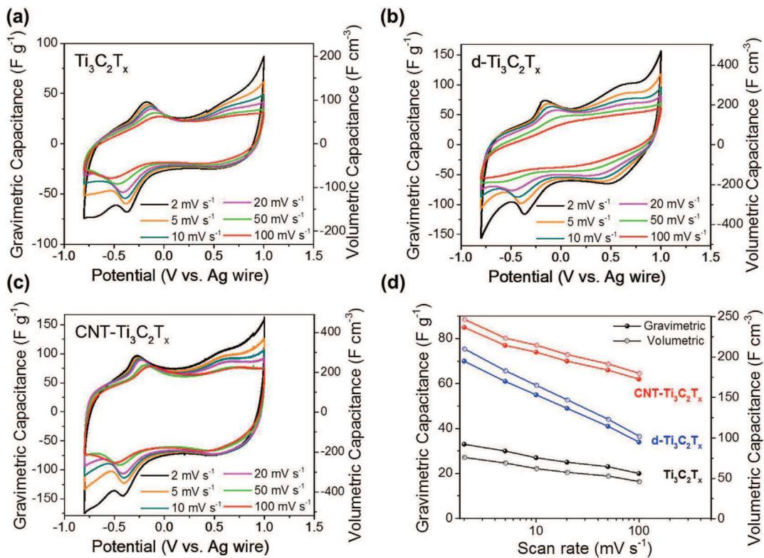
**Fig. 2.** Cyclic voltammograms of (a)  $\text{Ti}_3\text{C}_2\text{T}_x$ , (b)  $\text{d-Ti}_3\text{C}_2\text{T}_x$  and (c)  $\text{CNT-Ti}_3\text{C}_2\text{T}_x$  in 1M EMITFSI in acetonitrile electrolyte at different scan rates and (d) summary of the change of capacitance with the potential scan rate. These measurements were done using a three-electrode Swagelok cell.
