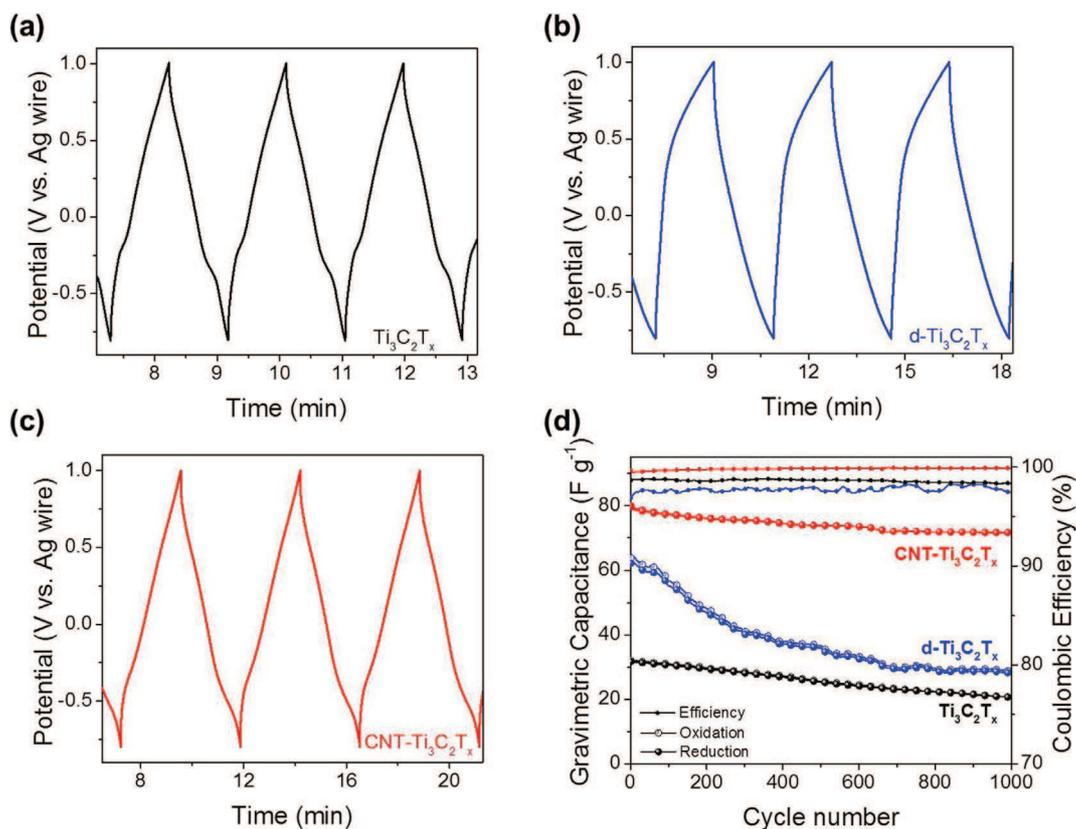
**Fig. 4.** Galvanostatic charge–discharge curves of (a)  $\text{Ti}_3\text{C}_2\text{T}_x$ , (b)  $\text{d-Ti}_3\text{C}_2\text{T}_x$  and (c)  $\text{CNT-Ti}_3\text{C}_2\text{T}_x$  in 1M EMITFSI in acetonitrile electrolyte obtained at  $1 \text{ A g}^{-1}$  and (d) the corresponding cycle life of those electrodes. These measurements were done using a three-electrode Swagelok cell.
