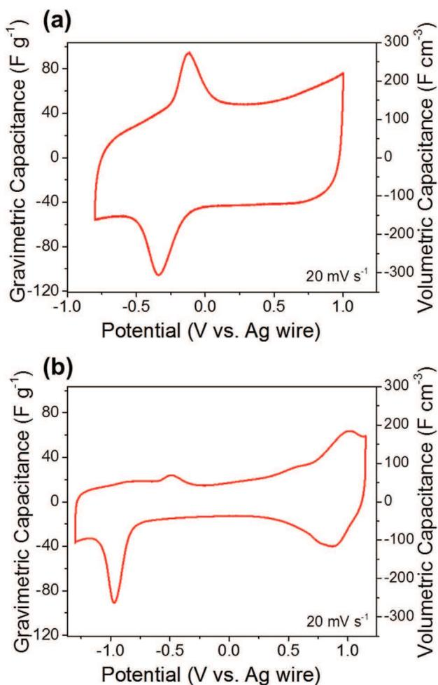
**Fig. 7.** Cyclic voltammetry of CNT-Ti<sub>3</sub>C<sub>2</sub>T<sub>x</sub> at 20 mV s<sup>-1</sup> in 1 M solutions of EMIBF<sub>4</sub> (a) and TEABF<sub>4</sub> in acetonitrile (b).
