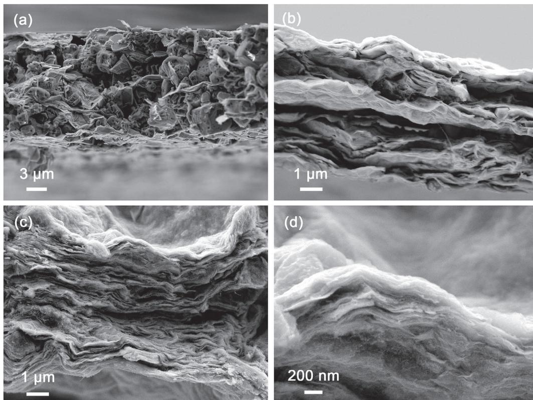
**Fig. 1.** Scanning electron microscope images of (a) rolled  $\text{Ti}_3\text{C}_2\text{T}_x$  "clay", (b)  $\text{d-Ti}_3\text{C}_2\text{T}_x$  and (c–d)  $\text{CNT-Ti}_3\text{C}_2\text{T}_x$  electrode films.
