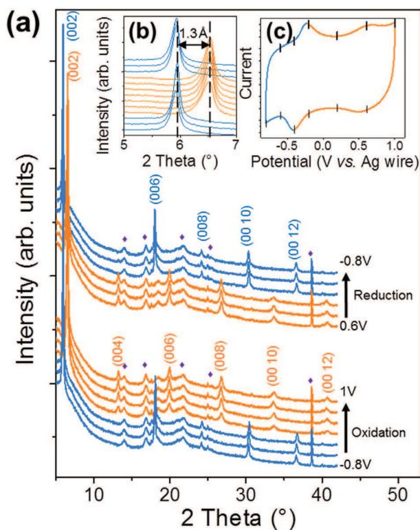
**Fig. 5.** In-situ XRD patterns of  $\text{CNT-Ti}_3\text{C}_2\text{T}_x$  at different potentials in the  $5\text{--}42^\circ$   $2\theta$  range. Purple diamonds indicate peaks coming from the cell for *in situ* measurements. Inset (b) shows a zoom in the  $5\text{--}7^\circ$   $2\theta$  range and (c) CV recorded at  $20 \text{ mV s}^{-1}$ . (For interpretation of the references to color in this figure legend, the reader is referred to the web version of this article.)
