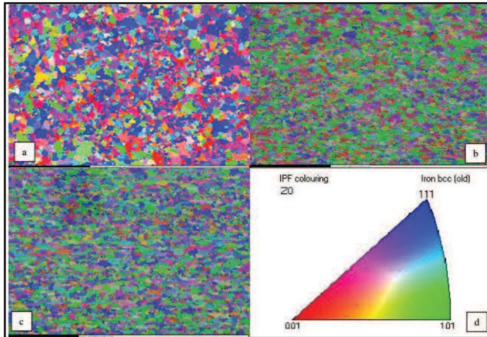
**Figure 9:**Crystallographic orientation plans for the DP 780. (a): Upper surface before air bending. (b): Thickness surface before air bending. (c): Thickness surface after air bending up to 30 degrees. (d): Legend indicating the Miller indices: crystallographic orientations.
