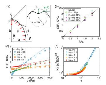
FIG. 2 (color online). Indentation at the pole. (a) Schematic of a deformed ellipsoidal specimen. (b) Dependence of GIR  $K/K_s$ on b/a for four different elastic polymers and p = 0. (c) GIR  $K/K_s$ , as a function of the internal pressure p for four aspect ratios  $b/a = \{0.5, 1, 1.5, 2\}$  and E = 1 MPa. (d) Dimensionless experimental rigidity  $Kl_b^2/D$  against dimensionless pressure  $\tau$ .
