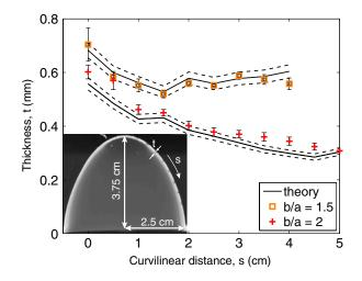
FIG. 4 (color online). Comparison between measured and predicted thickness profile for two unpressurized shells with b/a =1.5 and 2 and 0.9 < E < 1 MPa. Solid and dashed lines represent mean value ± standard deviation for the predicted thickness. (Inset) Scanned image of a shell with aspect ratio b/a = 1.5 cut in half.
