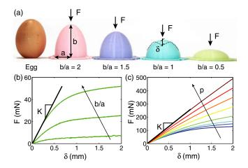
FIG. 1 (color online). (a) A chicken's egg and 500  $\mu$ m thick ellipsoidal shell samples with four aspect ratios  $b/a = \{2, 1.5, 1, 0.5\}$  and four elastomers with Young's modulus  $E = \{0.2, 0.5, 0.6, 1\}$  MPa. (b) Load-displacement curves for indentation at the pole for an in-out differential pressure p = 0 Pa, E = 1 MPa, and three different aspect ratios b/a = 0.5, 1, and 2. (c) Load-displacement curves for indentation at the pole for b/a = 1.5, E = 1 MPa, and 0 kPa.
