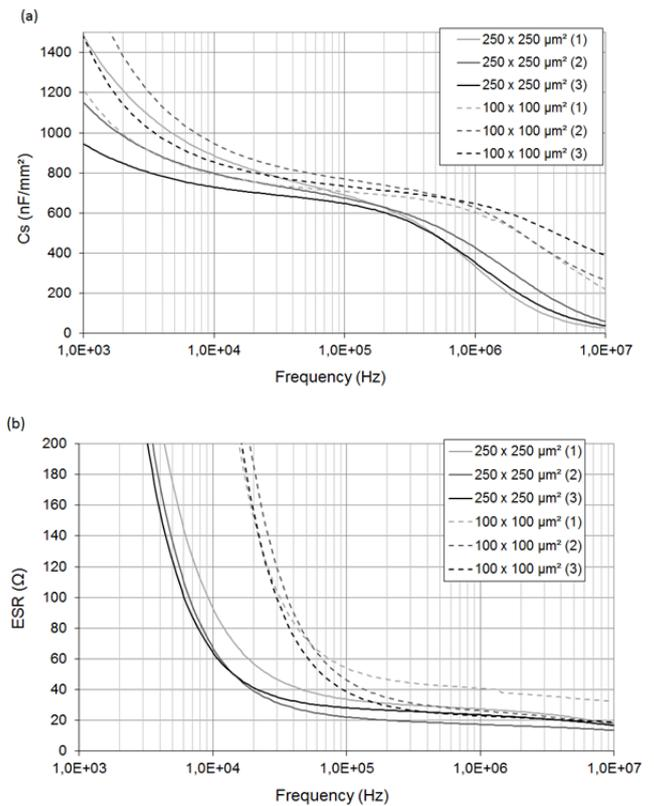
**Figure 4.** Measured a) specific capacitance and b) equivalent series resistance versus frequency for  $250 \times 250 \mu\text{m}^2$  and  $100 \times 100 \mu\text{m}^2$  3D capacitors fabricated with electrochemical etching method. Density is 1 pore/ $\mu\text{m}^2$
