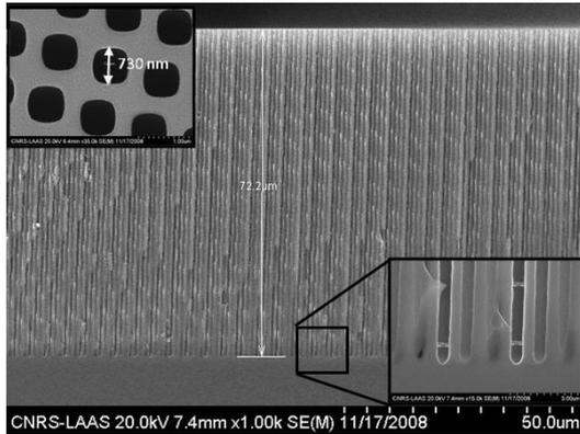
**Figure 3.** SEM pictures of array with a density of 1 pore/ $\mu\text{m}^2$  after 3h of electrochemical etching with a zoom on the bottom of the pores; insert: top view where pore width is shown to be 730 nm.
