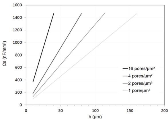
Figure 2. Specific capacitance versus depth ( $h$ ) for 4 different pore densities. Pores are arranged in hexagonal arrays with  $w = \frac{3}{4} p$ . Dielectric in this case is ON ( $\text{SiO}_2$  5 nm/ $\text{Si}_3\text{N}_4$  10 nm)
