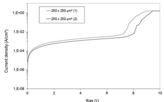
**Figure 5.** Measured current density versus bias for two  $250 \times 250 \mu\text{m}^2$  3D capacitors fabricated with electrochemical etching method.
