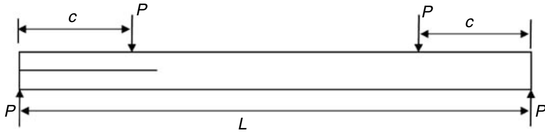
Figure 11. Specimen under pure mode II loading condition.
