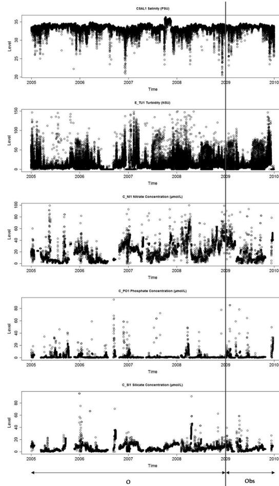
Fig. 5. Five completed MAREL-Carnot signals from 2005 to 2009 by mobile average: C\_SAL1, E\_TU1, C\_NI1, C\_PO1, C\_SI1. Vertical line separates data into 2 subsets. Subset **O** corresponds to 2005-2008 period which is used for HMM building. Subset **Obs** relates to the year 2009 which is used for generalisation and accordingly does not participate in HMM building.
