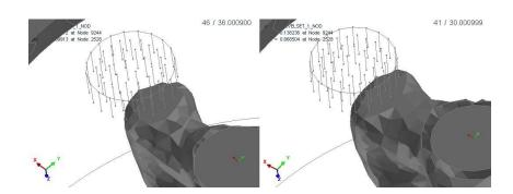
FIGURE 28. Comparison between the final designs without (left) and with (right) friction for Example 15. Remark that the shape of the foot is larger when friction is present.
