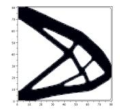
FIGURE 6. Final design for Example 1-2bis
