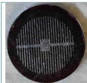
Figure 2.  $\text{CsI-GeSe}_2\text{-Ga}_2\text{Se}_3$  glass source with Al front electrodes.
