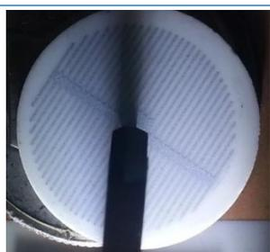
Figure 5.  $\text{Rb } \beta'' \text{ alumina}$  source and spring contact.
