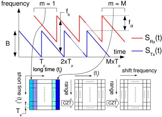
Fig. 2: Instantaneous frequency over  $M$  transmitted ramps
