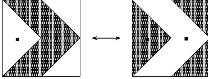
Figure 2: Two period cells of an interchangeable material with a herring-bone pattern.
