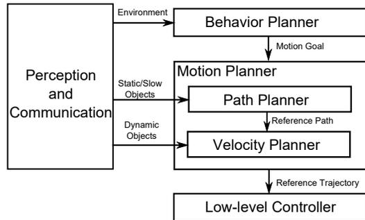
Fig. 2: Autonomous driving architecture: a simplified view
