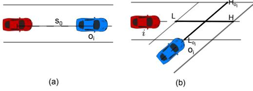
Fig. 6: (a) Obstacle following. (b) Intersection.
