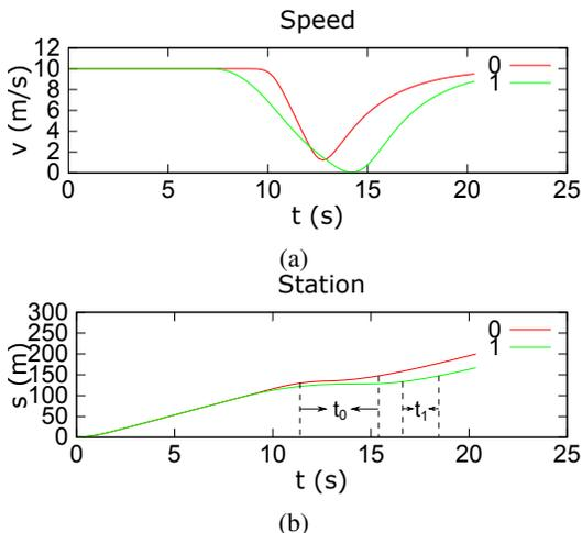
Fig. 9: Vehicle 0 has priority while vehicle 1 does not. Vehicle 0 performs an emergency brake from 11s to 13s. (a) Speed profiles of two vehicles. (b) Station of two vehicles.  $t_0$  and  $t_1$  are respectively two intervals that two vehicles are in the intersection. We note that two intervals do not overlap.
