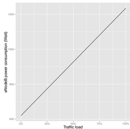
Fig. 1. Power consumption of a 4G base station.
