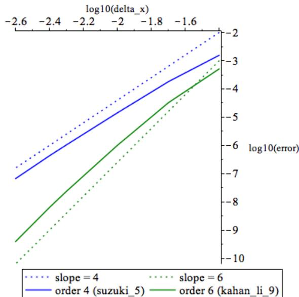
Figure 2: Convergence study for palindromic methods at order 4 (blue, Suzuki scheme) and 6 (green, Kahan-Li scheme) with high CFL number  $\beta = 50$ . The dotted lines are reference lines with slopes 4 and 6 respectively. We observe that the schemes are stable and that for sufficiently fine meshes, the expected rates of convergence are attained.
