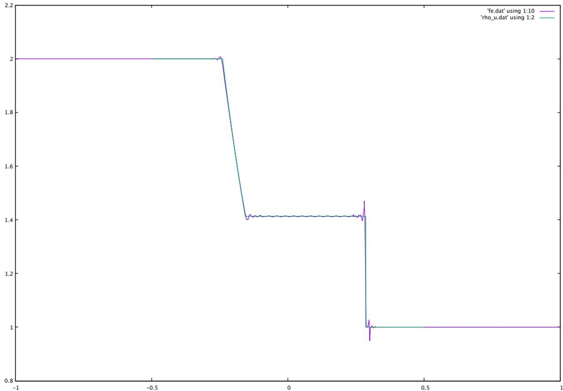
Figure 3: Riemann problem with  $\tau = 0$ . Comparison of the exact density (green curve), and the numerical sixth-order solution with complex time steps (purple curve). The number of DG cells is  $N_x = 100$  and the CFL number  $\beta = 3$ .
