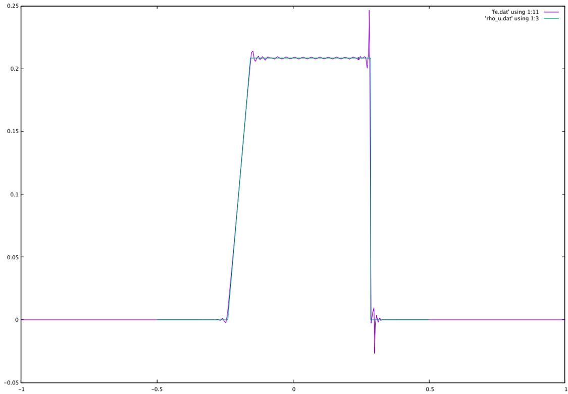
Figure 4: Riemann problem with  $\tau = 0$ . Comparison of the exact velocity (green curve), and the numerical sixth-order solution with complex time steps (purple curve). The number of DG cells is  $N_x = 100$  and the CFL number  $\beta = 3$ .
