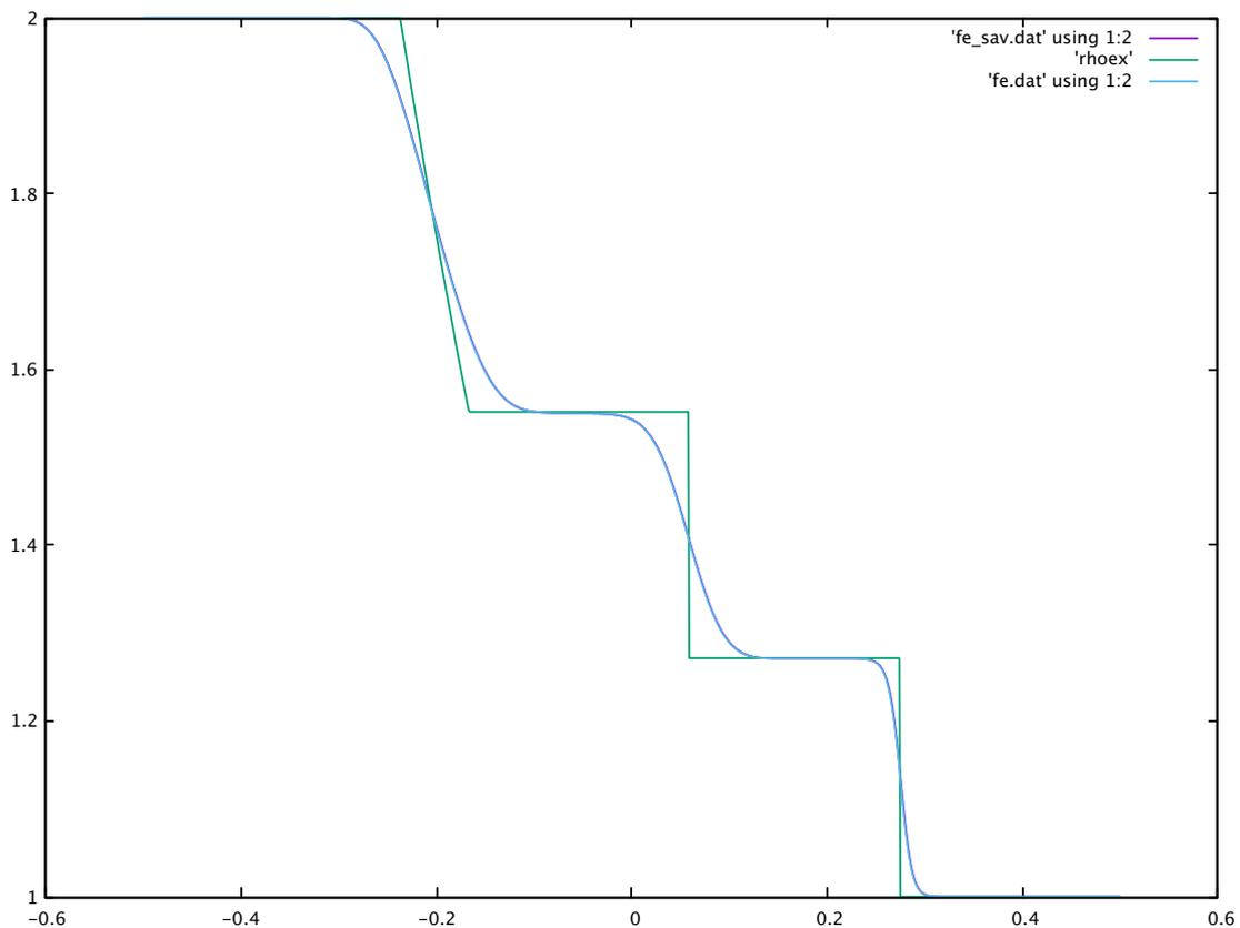
Figure 7: Riemann problem with  $\tau = 0.000519$ . Comparison of the exact density of the inviscid case (green curve), and the sixth-order complex numerical solution with  $\tau > 0$  (blue and purple curves: indistinguishable). The number of DG cells is  $N_x = 100$  or  $N_x = 1000$  and the CFL number  $\beta = 5$ . The relaxation parameter has the same effect as a viscosity parameter.
