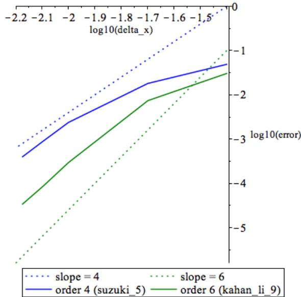
Figure 6: Convergence study for the low Mach test case with a CFL number  $\beta = 100$ . Comparison of the fourth-order Suzuki scheme (blue) and the sixth-order Kahan-Li scheme (green). The dotted lines are reference lines with slopes 4 and 6 respectively. We observe the expected convergence rates for fine enough meshes. With this CFL number, the schemes with complex time steps are unstable.
