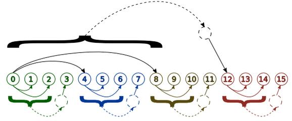
**Figure 4.** Representation of the transport links of the bi-scale model. In black, the upper scale system, while the colored systems are the lower scale systems. Numbers are the chord indexes in the initial sequence.
