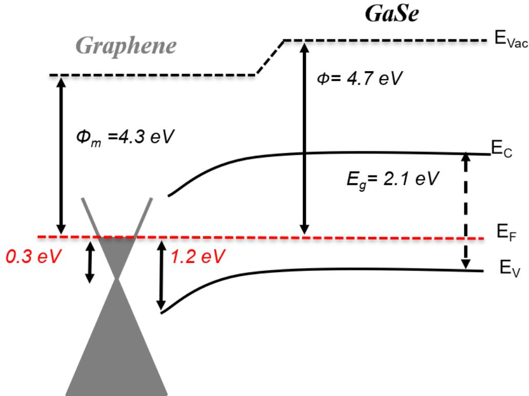
**Figure 6:** Schematic of the GaSe/Graphene band alignment diagram, as determined by XPS core level analysis.  $\Phi$  and  $E_F$  denote the work function and the Fermi energy, respectively.  $E_g$  is the energy gap.
