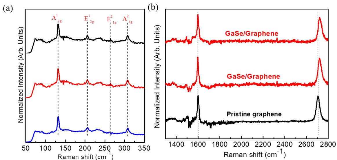
**Figure 3:** a) The characteristic peaks for different locations on GaSe grown on graphene, the spectra are exactly the same indicating substrate-independent growth with similar crystal quality owing to the vdW of 2D materials; b) Comparison of micro-Raman spectra taken on the pristine graphene (black color) and GaSe/graphene (red color) layers on different locations of the sample.
