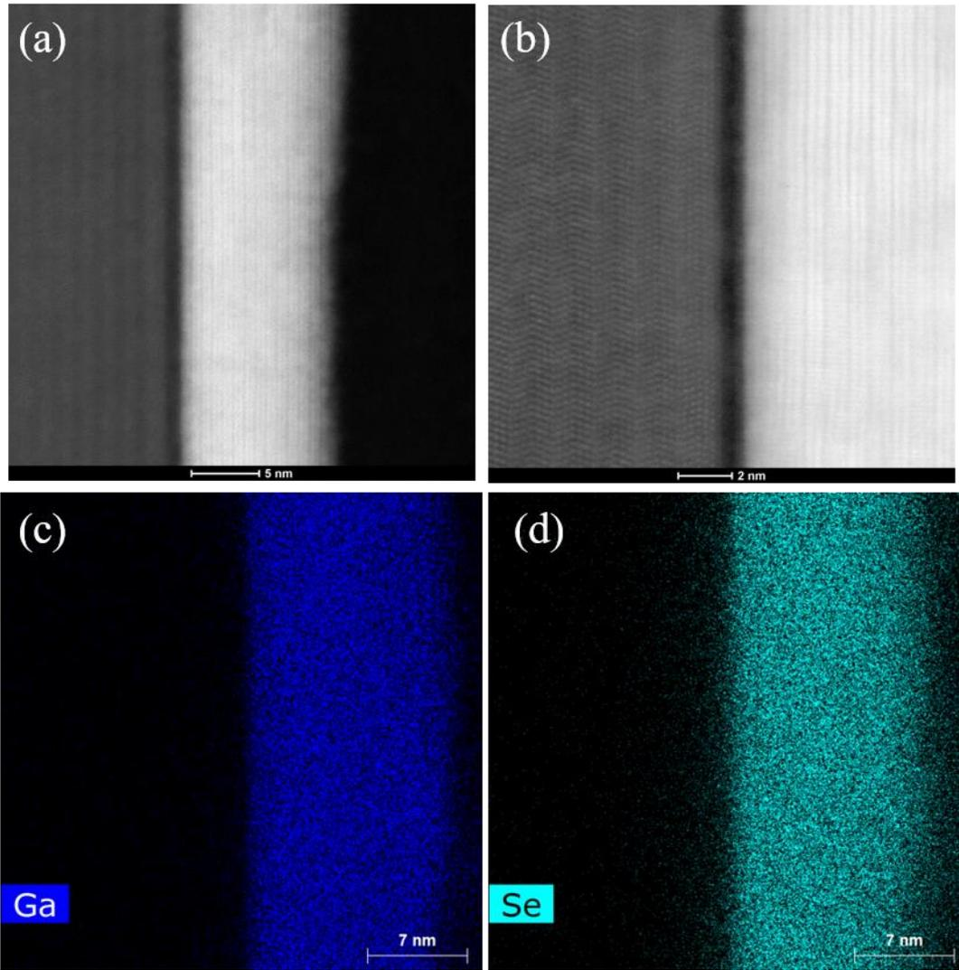
**Figure 2:** (a) and (b) Bright-field Scanning Transmission Electron Microscopy (STEM) image of GaSe/graphene heterostructure, high resolution STEM image place in the inset, the (c) (d) EDX elemental maps showing the spatial distribution of Ga and Se, respectively.
