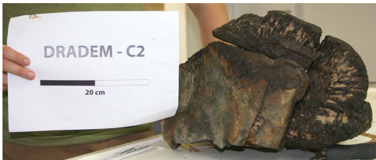
Figure 47: Reconstruction of the block DRA-C2-1. A crust follows the block on two sides. The crust is thicker on the right side, which may have been the upper side on the outcrop. There is no crust on two sides of the block, where it should be fixed on the outcrop.
