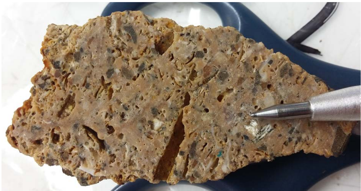
Figure 56: Section in the sedimentary matrix of the breccia (DRA-E1-7).
