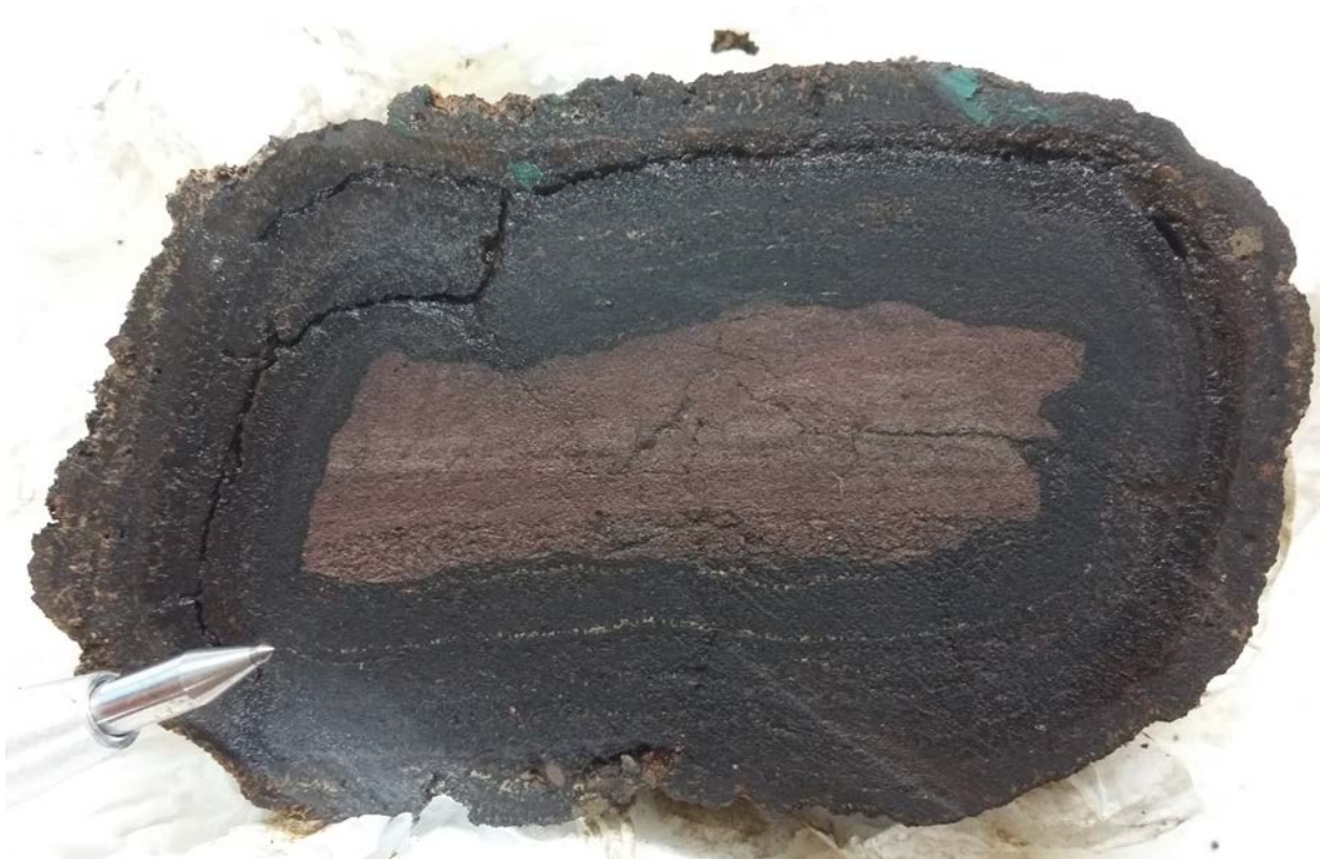
Figure 58: Sedimentary clast (claystone) in a nodule (DRA-E1-8).
