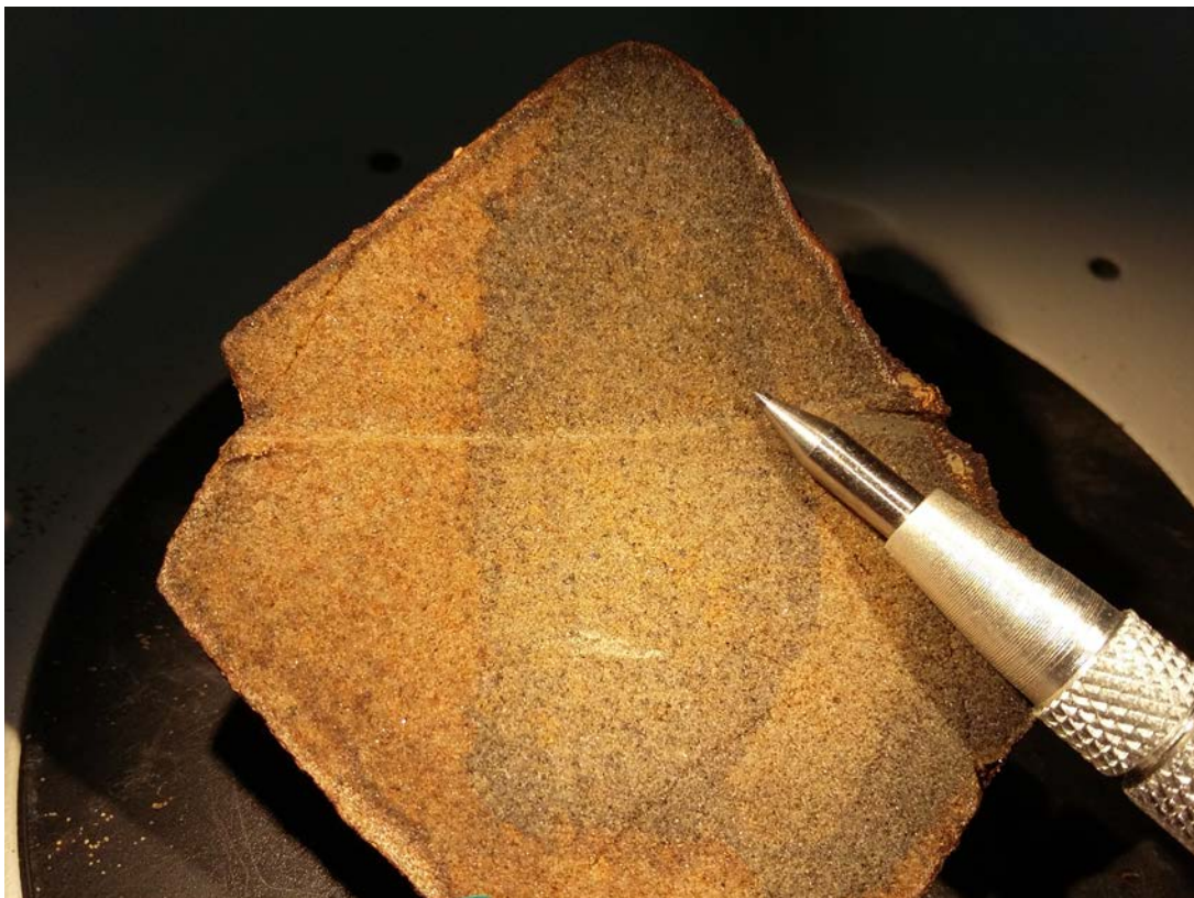
Figure 25: Section of sample DRA-G2-2: fine sandstone.
