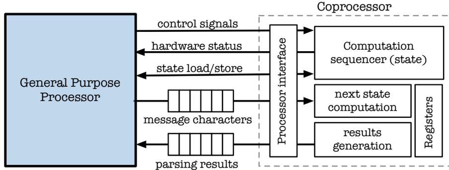
Fig. 6. Processor coupling with the protocol message parsers
