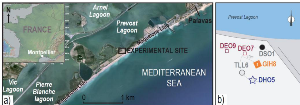
Fig. 1. Geographical location (a) of the Maguelone experimental site along the Gulf of Lion margin. Field spread (b). The monitoring system includes the TLL6 hole for time-lapse induction and sonic logging, downhole electrical resistivity observatories (in DEO7 and DEO9 holes), a downhole hydrochemical observatory (DHO5), a downhole seismic observatory (DSO1), a gas injection hole (GIH8).
