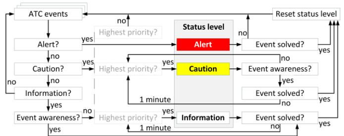
Figure 3. ATC event attention flow to determine working order and display presentation [84]
